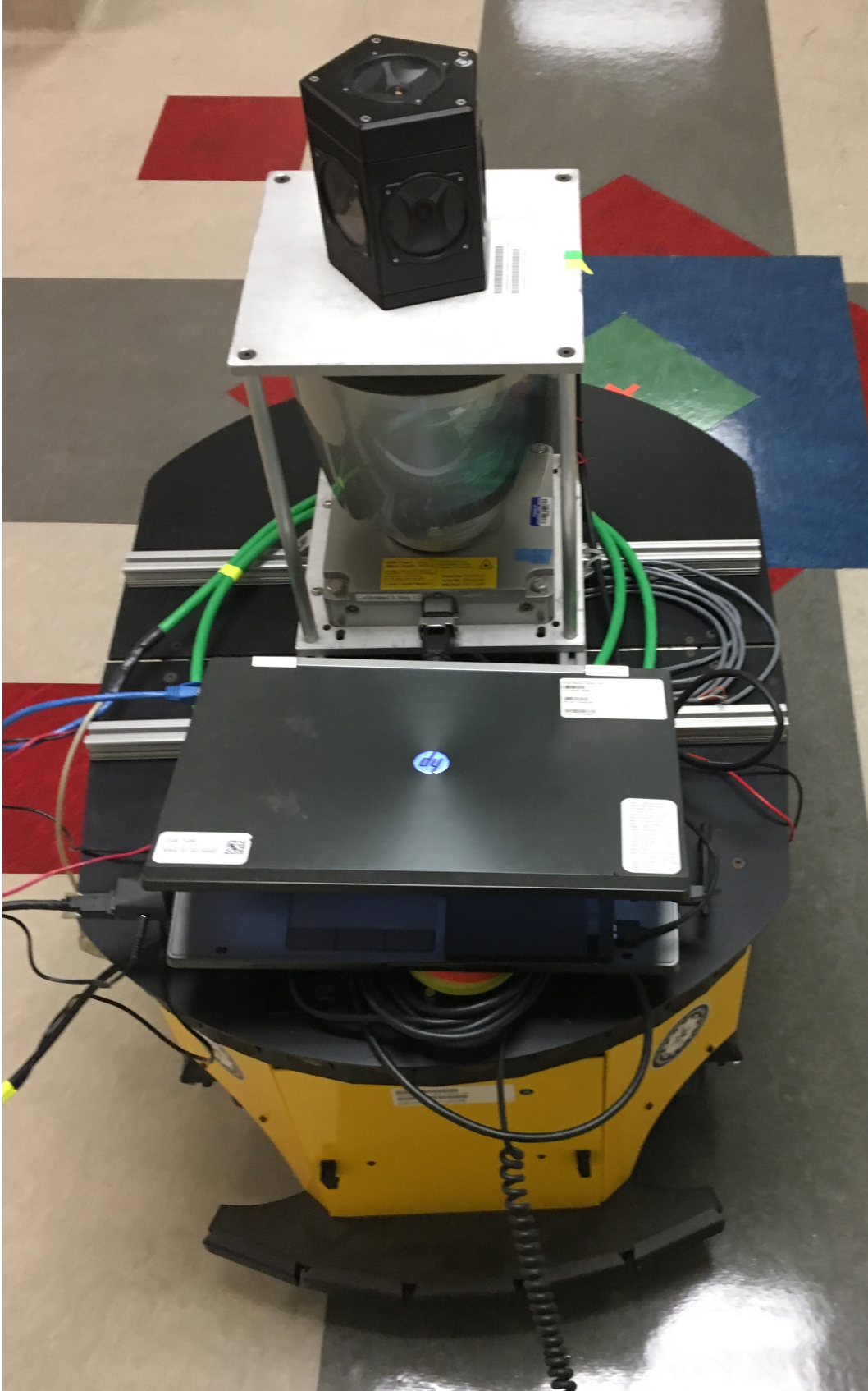
Figure 13: Camera and LIDAR platform on motorized ground vehicle.
