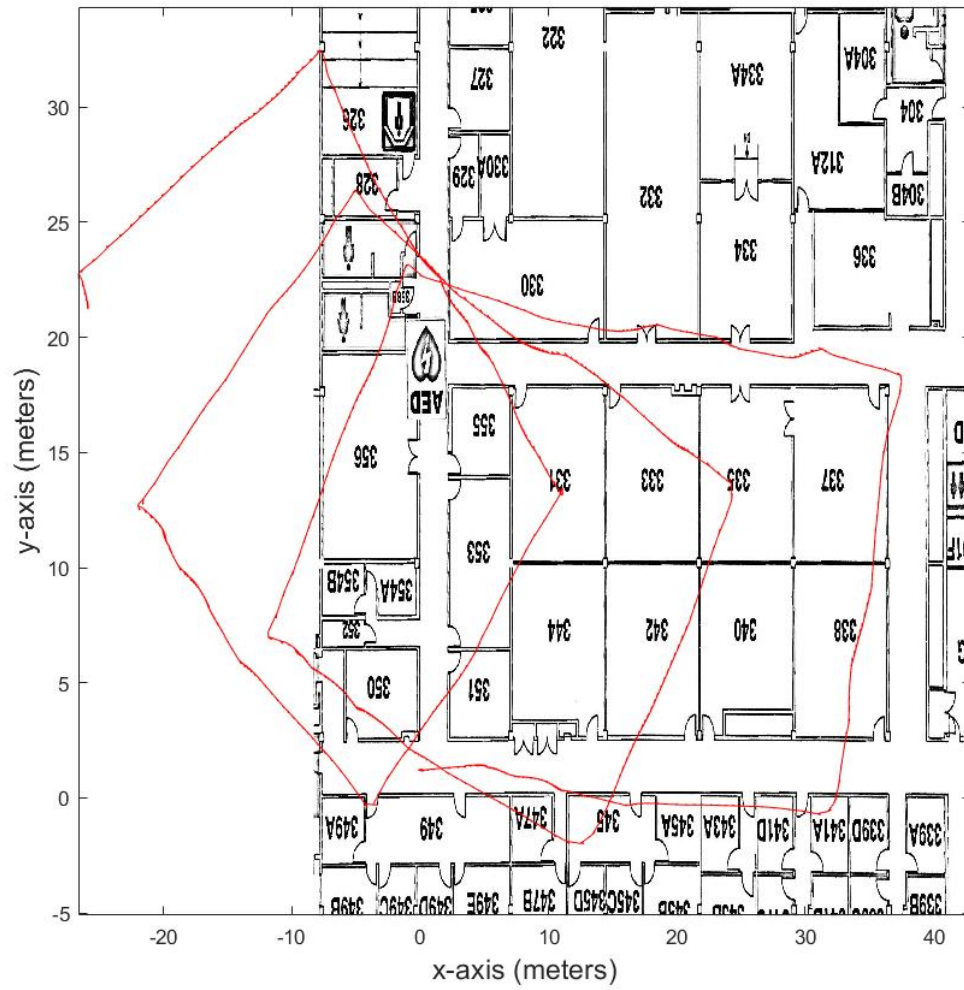
Figure 41: Plot of platform odometry in GTSAM without covariance.
