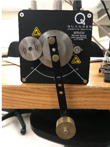
Fig. 8 An asymmetrical load is added to the motor system in Fig. 4 to evaluate the effectiveness of the adaptive control as shown in Figs. 9 and 10
