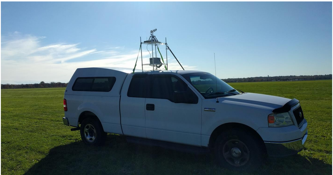
Figure 33. localizer mounted in the configuration used to collect data during experiment
