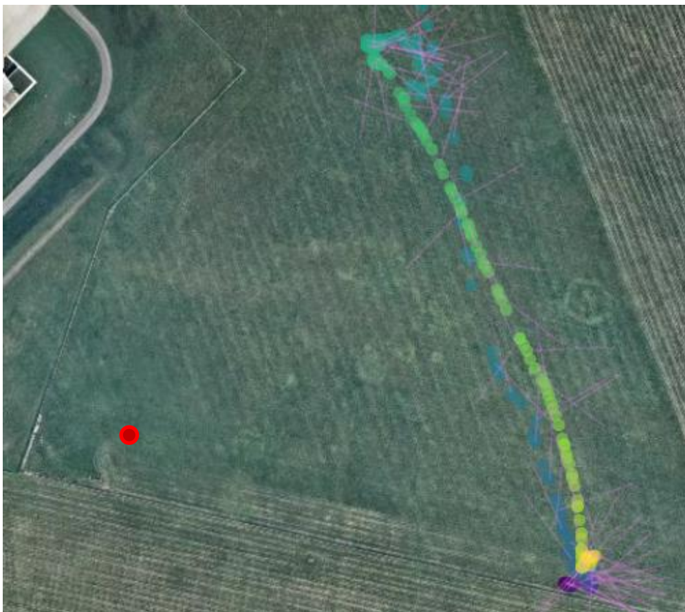
Figure 61. skyport telemetry history of the skypie on the 300 m line test, with the purple lines indicating the direction the sensor is facing at the time. The red dot indicates the location of the targets.
