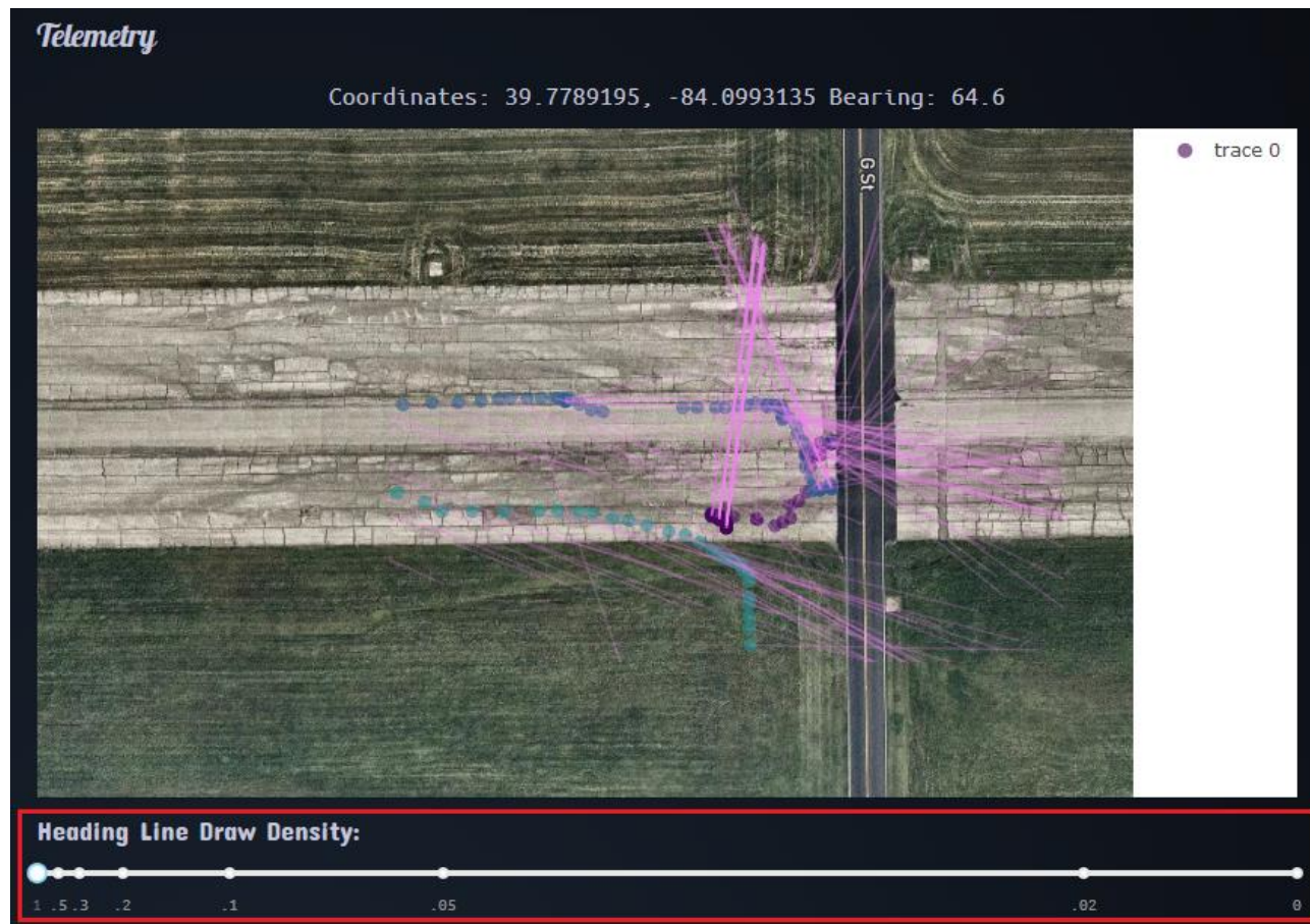
Figure 18. View history of compass heading 'Heading Line Draw Density' value slider. Each purple ray extends from a coordinate in time and indicates which way the sensor was facing. In this example, the antenna is mounted to a bicycle doing a half-circle.
