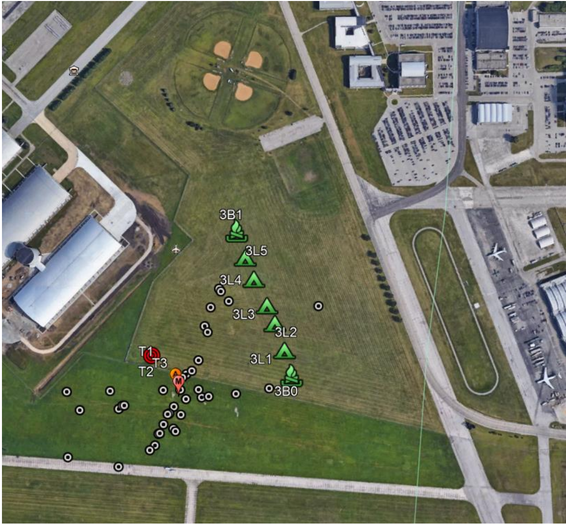
Figure 56. Guesses, median (red 'M' marker), and average (orange 'A' marker) coordinate predictions on 300 m line using centroid calculations
