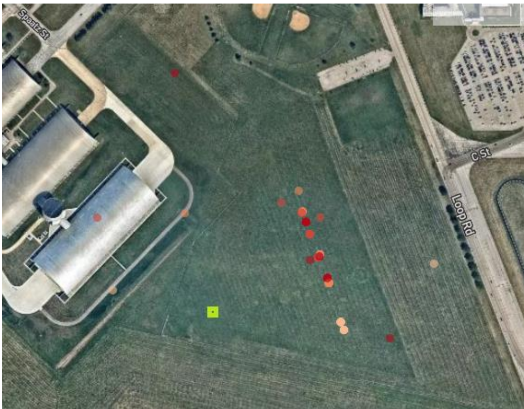
Figure 62. skyport geolocation predictions (circles) of targets (true location at green square) on the 300 m line
