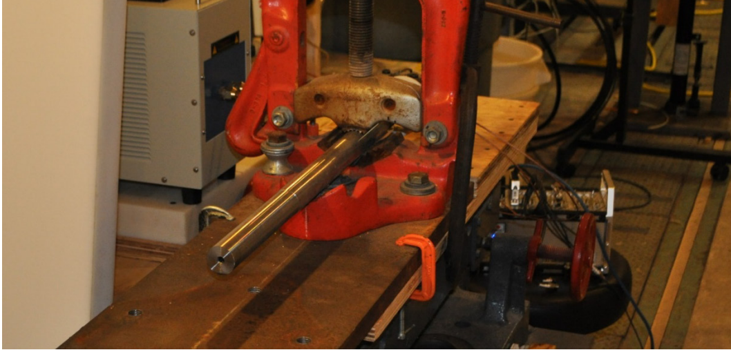
Fig. A-1 Mounted test barrel
