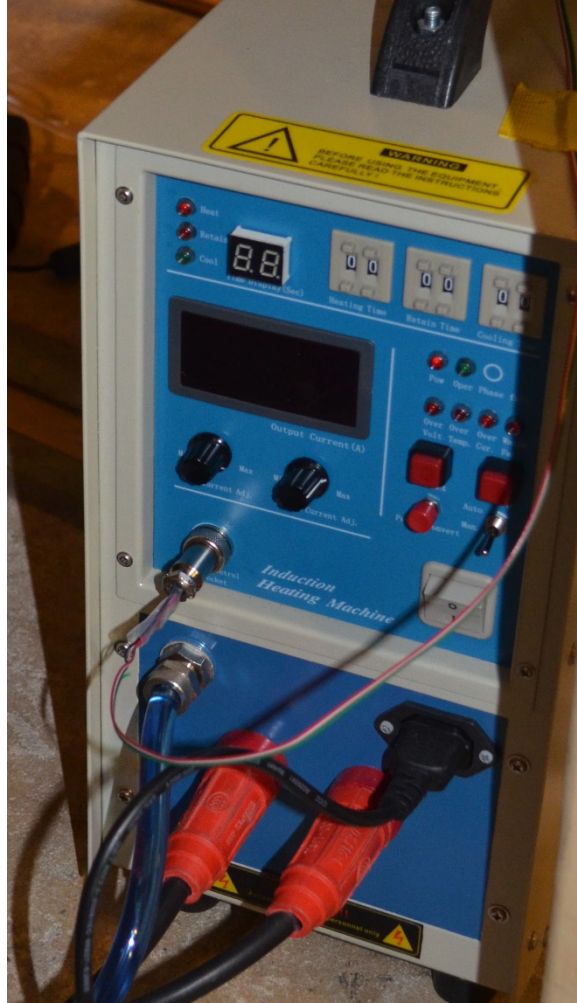
Fig. A-7 Induction furnace control panel
