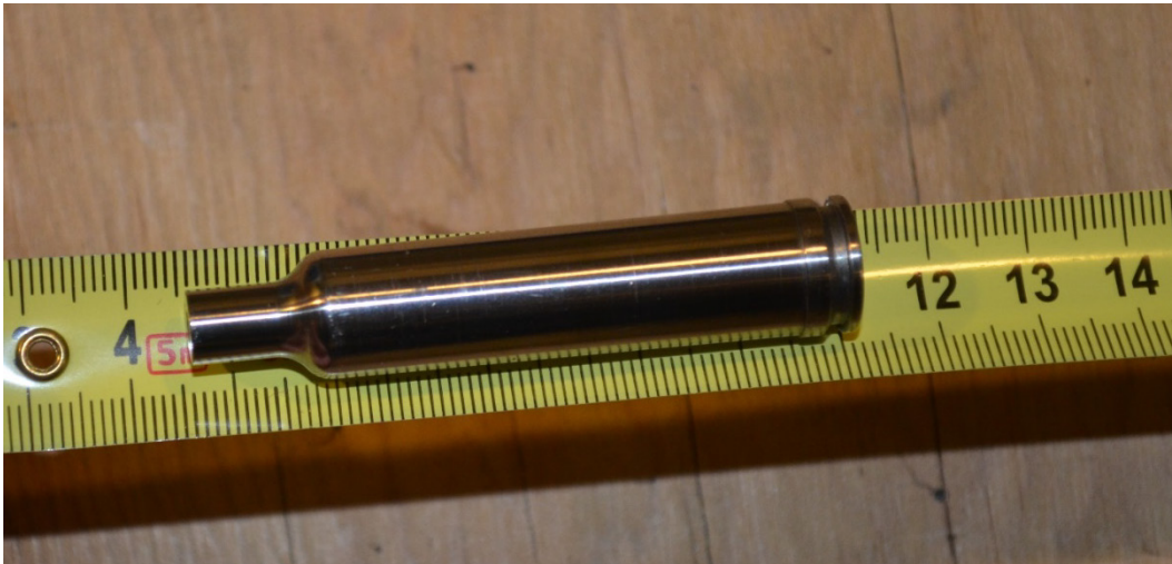
Fig. A-6 Chamber adaptor, used for reducing ullage with light propellant charges. Numbered scale is in centimeters.
