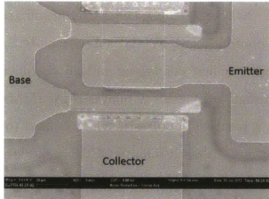
Figure 3-1: SEM image of the top view of a fabricated device
