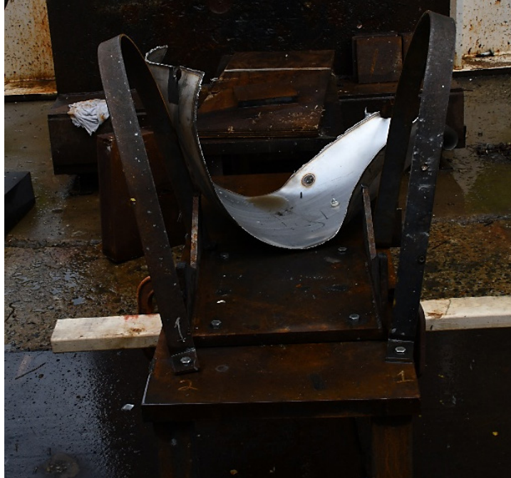
Fig. 40 EFP engagement postevent damage of the tank bindings with debris for the 75% fill 3/16-inch-thick stainless steel tank
