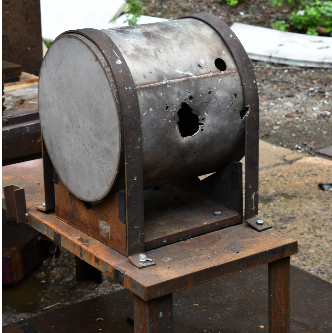
Fig. 38 EFP engagement postevent damage of a 3/16-inch stainless steel walled tank, entrance hole
