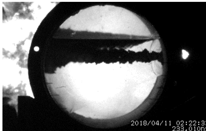
Fig. 15 High-speed video screen capture (side view) of shaped charge jet at exit of a 3/16-inch-thick tank with 1/2-inch polycarbonate (transparent) endcaps 0.233 ms after detonation
