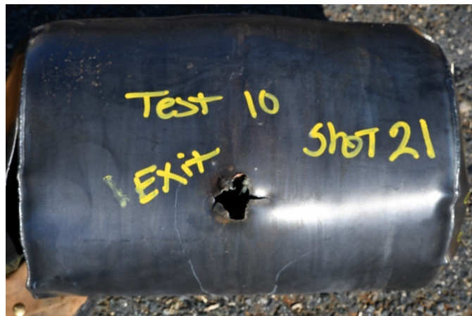
Fig. 32 1/16-inch steel tank with 20 layers of Kevlar wrap (removed), exit hole
