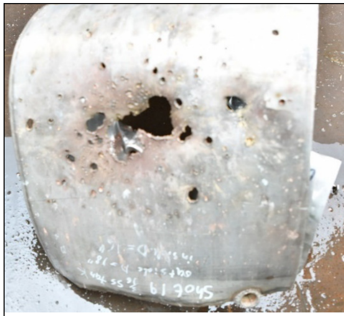
Fig. 42 Postevent, 75% filled double walled 3/16-inch stainless steel tank EFP engagement, EFP particle entry location
