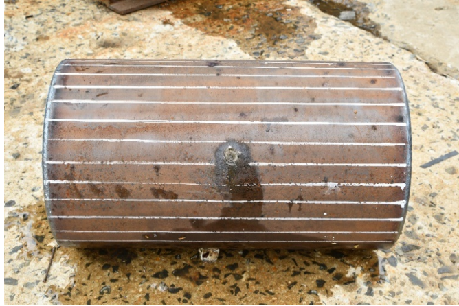
Fig. 14 Exit hole of 3/16-inch-thick fuel tank with double wrap of 1/2-inch inner Kevlar felt liner
