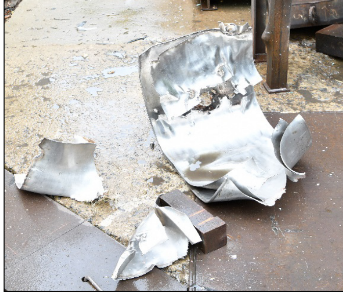
Fig. 43 Postevent, 75% filled double walled 3/16-inch stainless steel tank EFP engagement tank debris
