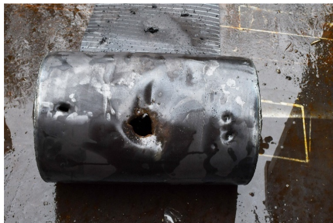
Fig. 25 Postevent photo of 1/16-inch-thick steel tank with 1/2-inch rubber outer wrap (removed), entry hole
