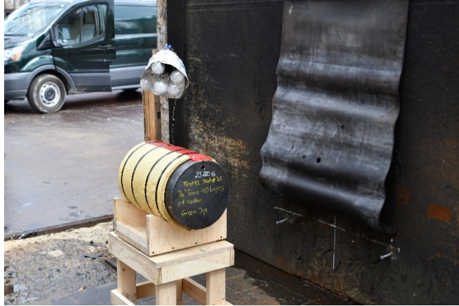
Fig. 27 1/16-inch-thick steel tank with 20-layer Kevlar overwrap (pre-event) on the experimental stand
