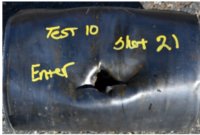
Fig. 31 1/16-inch steel tank with 20 layers of Kevlar wrap (removed), entrance hole
