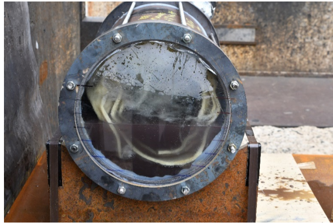
Fig. 20 Postevent photo of 3/16-inch-thick tank with Kevlar inner liner and 1/2-inch polycarbonate endcaps
