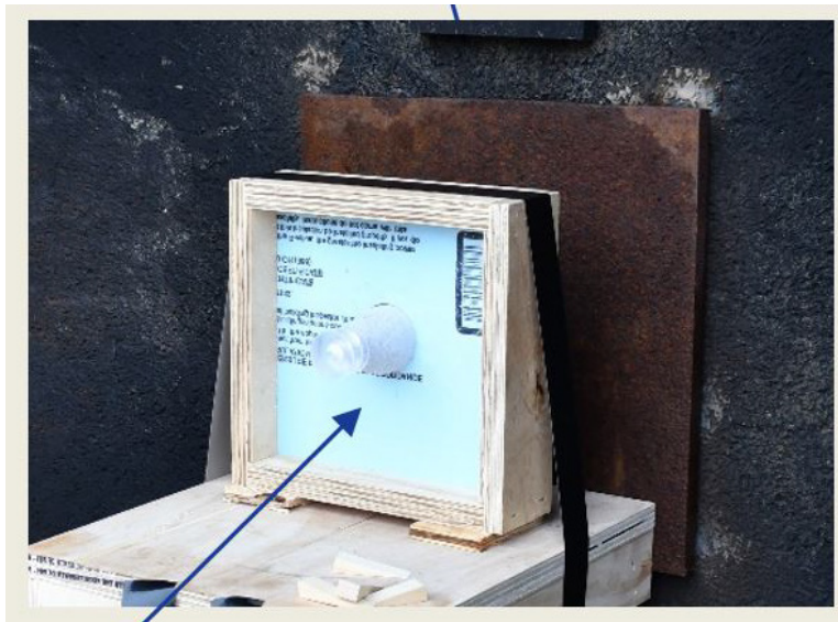
Fig. 4 Baseline setup showing 65-mm shaped charge jet warhead up range of blast wall
