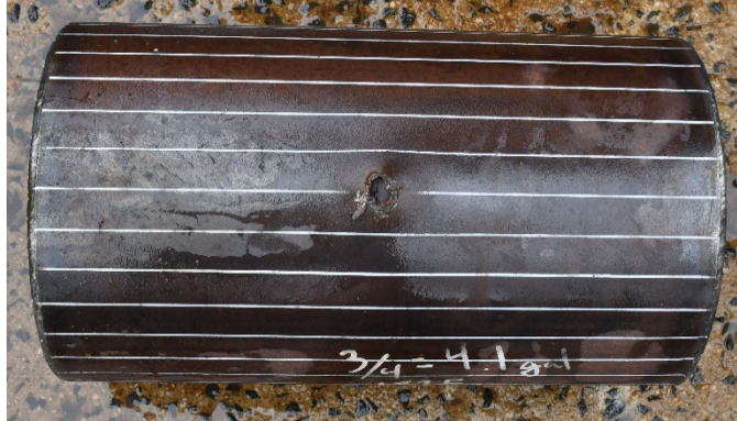
Fig. 11 Exit hole of 3/16-inch-thick fuel tank with double wrap of 1/4-inch inner rubber liner
