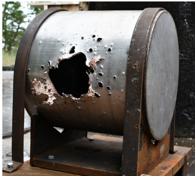
Fig. 37 EFP engagement postevent damage of a 3/16-inch stainless steel tank, exit hole
