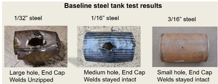
Fig. 8 Exit holes of 1/32-, 1/16-, and 3/16-inch-thick steel fuel tanks
