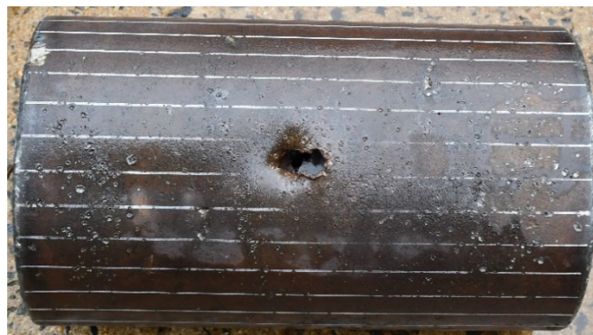
Fig. 10 Entry hole of 3/16-inch-thick fuel tank with double wrap of 1/4-inch inner rubber liner
