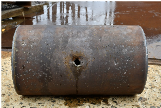
Fig. 13 Entry hole of 3/16-inch-thick fuel tank with double wrap of 1/2-inch inner Kevlar felt liner
