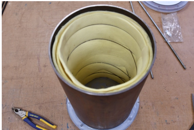
Fig. 17 Partial build view of 3/16-inch fuel tank with Kevlar inner liner and 1/2-inch polycarbonate endcaps
