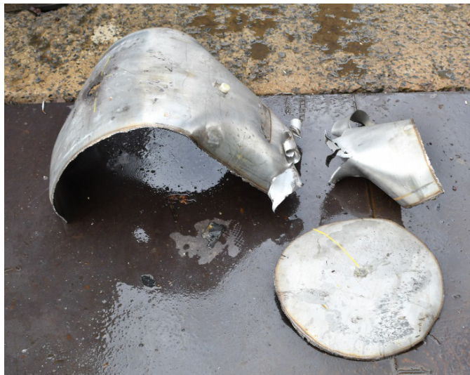
Fig. 39 EFP engagement postevent debris of a 75% filled 3/16-inch-thick stainless steel tank (note remains and the exit-hole location)
