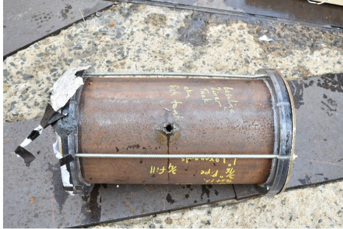
Fig. 16 Postevent photo of 3/16-inch-thick tank with 1/2-inch polycarbonate endcaps
