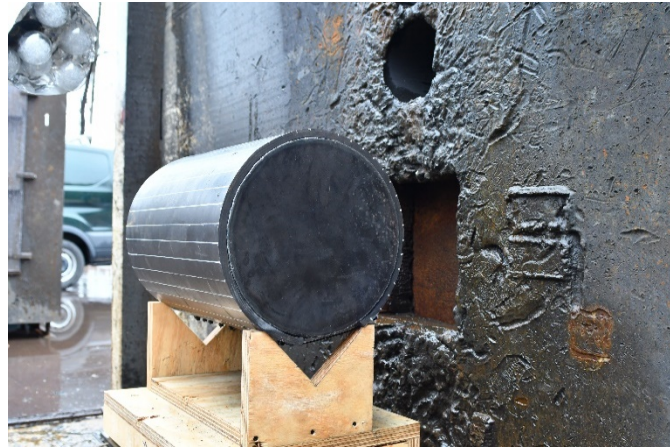
Fig. 21 1/16-inch-thick steel tank with 1/2-inch rubber overwrap (pre-event) on the experimental stand
