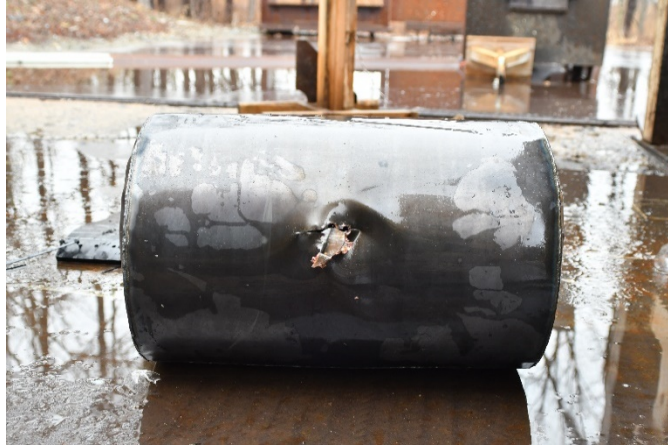
Fig. 26 Postevent photo of 1/16-inch-thick steel tank with 1/2-inch rubber outer wrap (removed), exit hole
