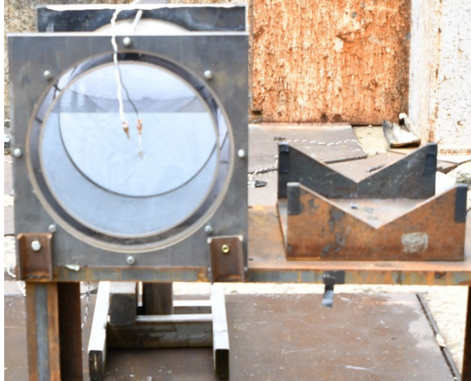
Fig. 41 Pre-event, 75% filled 3/16-inch stainless steel double walled tank with polycarbonate endcaps for EFP engagement experiment
