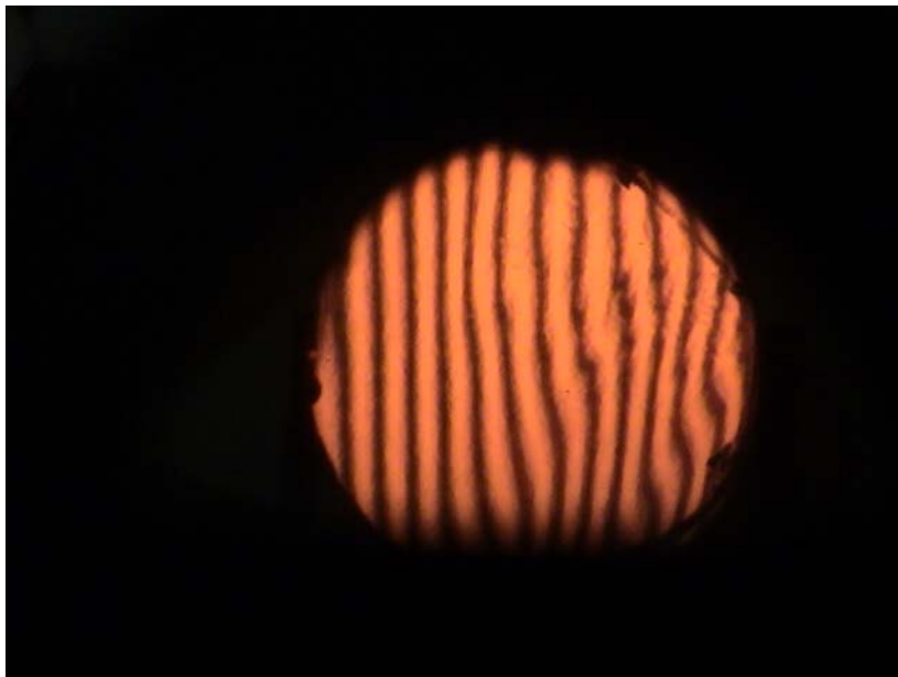
Figure 16. Distortion pattern example 5, lens rotated, unacceptable.
