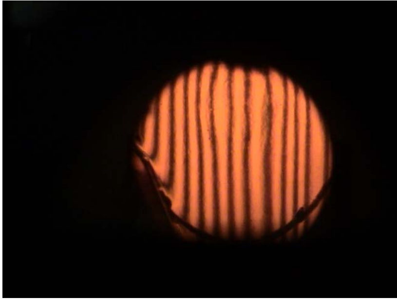
Figure 15. Distortion pattern example 4, “as worn” marginally acceptable.
