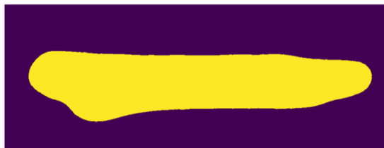
(e) The mask is calculated after closing the contour, removing small objects, and filling holes.
