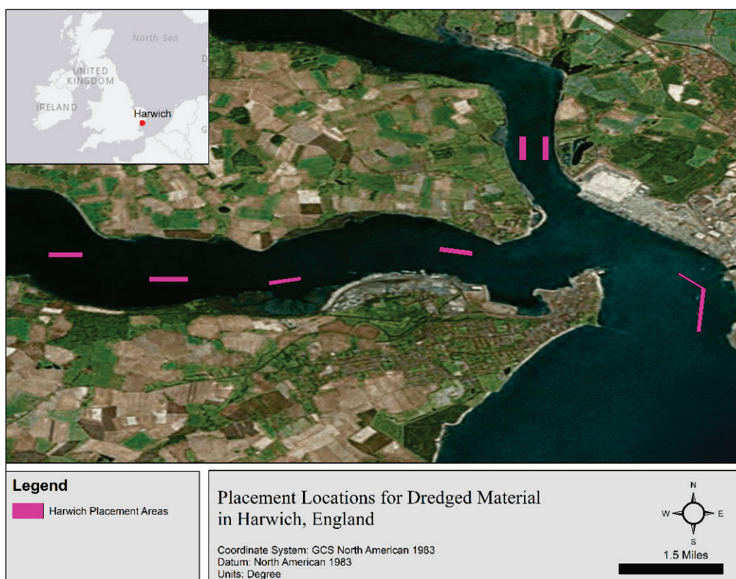
Figure 23. Subtidal placement locations for dredged sediment at Harwich Haven, England (data from Simpson et al. 2005), selected as part of the sediment replacement program.
