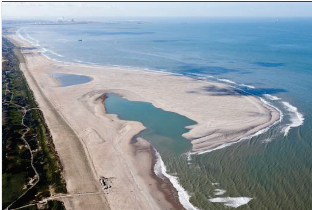
Figure 5. The Sand Engine demonstration project in The Netherlands, immediately after construction in 2011. Pools were intentionally designed for habitat.
