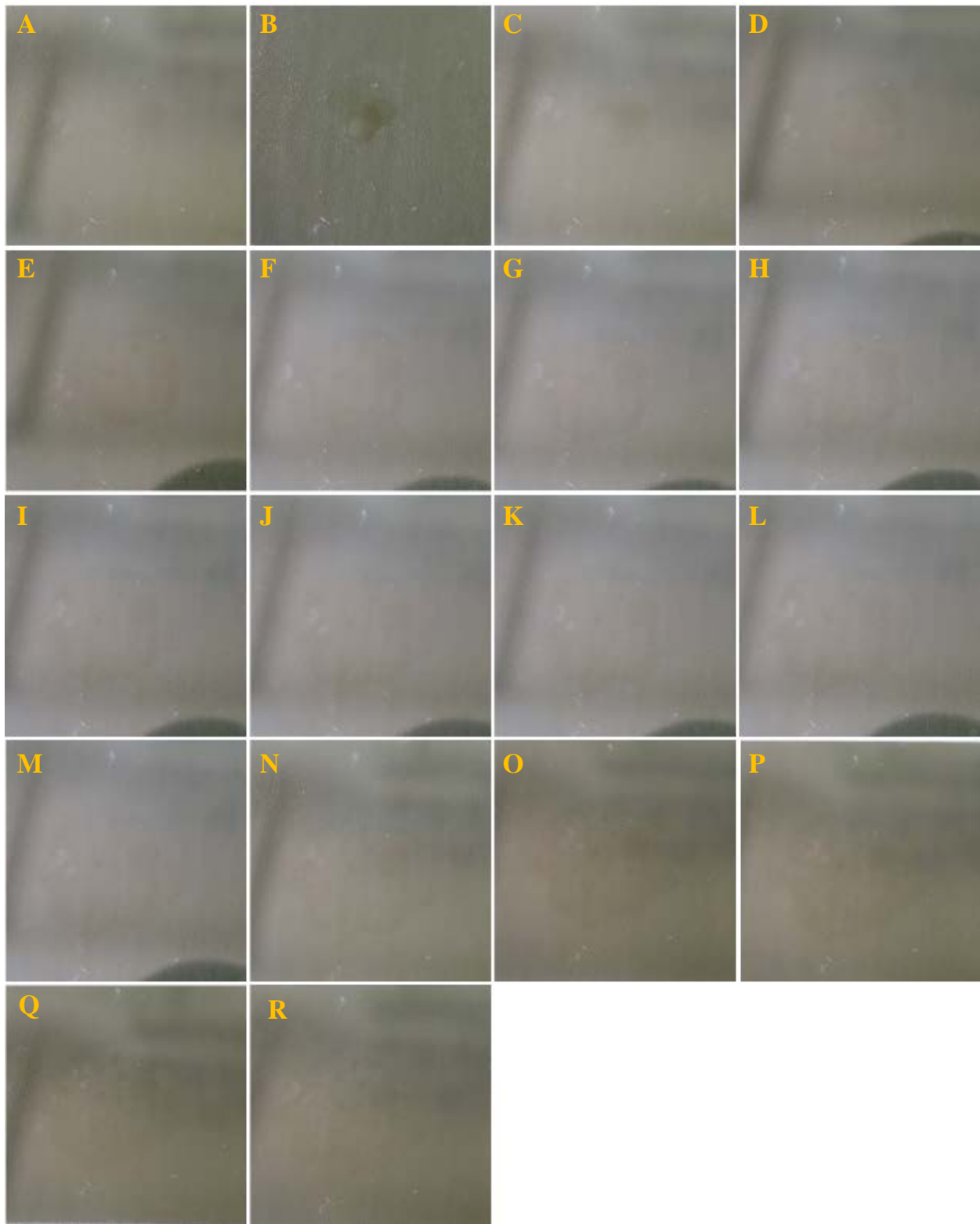
Fig. D1 — DFP on Fomblin Y oiled paint. Images of a coupon before application (A) and at 0 (B), 0.5 (C), 1 (D), 1.5 (E), 2 (F), 2.5 (G), 3 (H), 3.5 (I), 4 (J), 4.5 (K), 5 (L), 5.5 (M), 10 (N), 15 (O), 20 (P), 25 (Q), and 30 (R) min following application of the target. These images were collected with a glass cover in place to limit evaporation. Reflections from the cover can be seen in some images.
