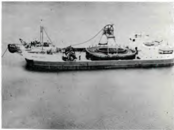
Figure B-3. Laying Sea End of Cable
