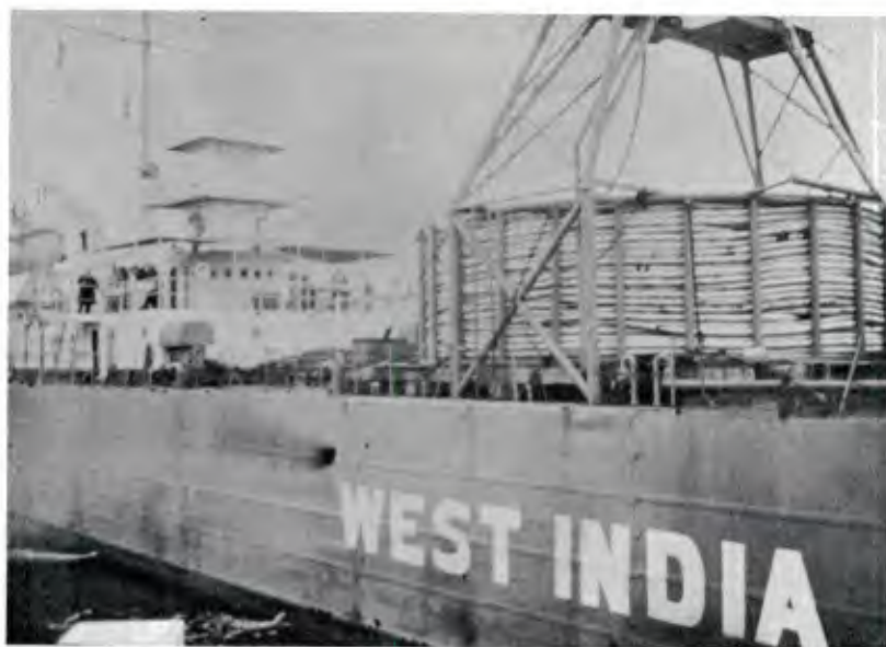
Figure 5-4. Deck Storage of Cable on Small Cable Layer
