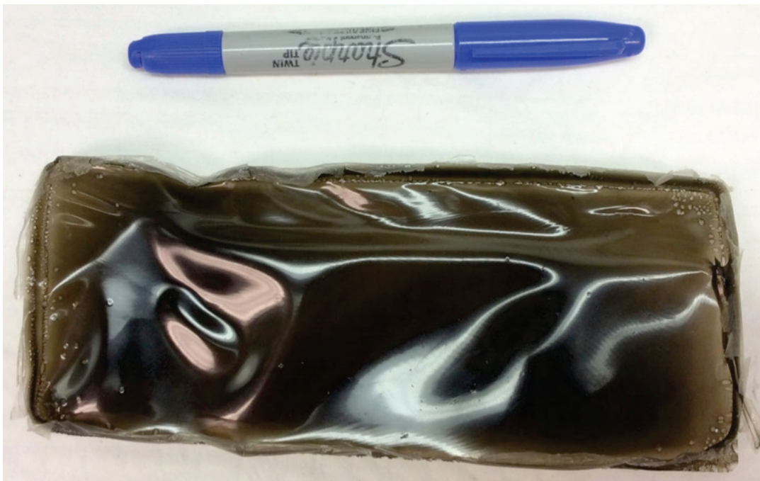
Figure 11. Dried diluted CSGO membrane after 72 hours of incubation.
