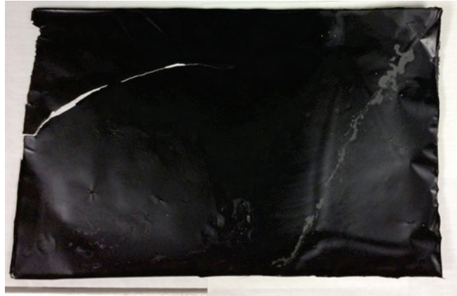
Figure 33. Scaled d-g-CSGO membrane.
