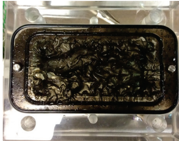
Figure 14. Top View of d-CSGO membrane after failure.
