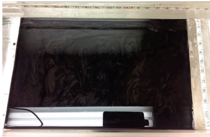
Figure 32. d-g-CSGO solution after pouring onto Plexiglass mold.
