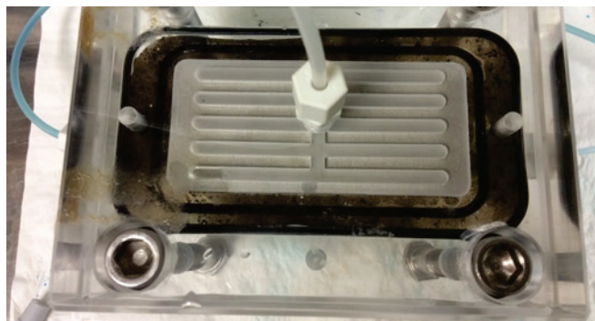
Figure 13. Membrane filtering MB (10 mg/000).
