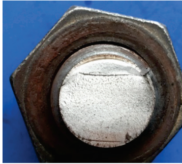
Figure 34. Fractographic profile of specimen #15 (Regular 10S_20T N=228736 ).
