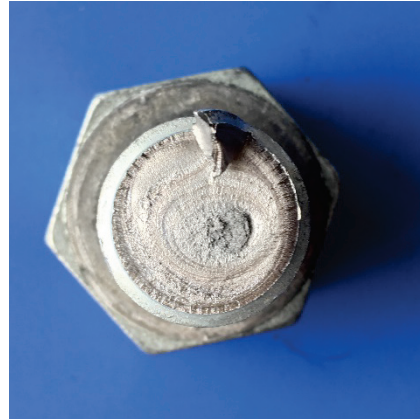
Figure 28. Fractographic profile of specimen #2 (Galvanized 20S_20T N=43,423 ).
