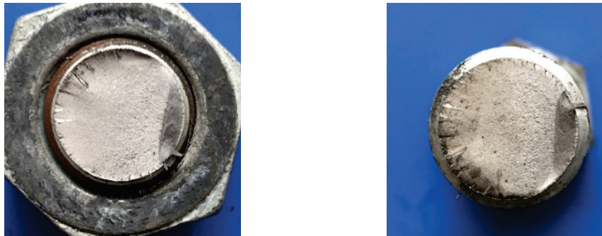
Figure 33. Fractographic profile of specimen #4 (Galvanized 10S_20T N=100,167).
