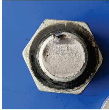
Figure 30. Fractographic profile of specimen #6 (Galvanized 16S_16T N=32,964 ).
