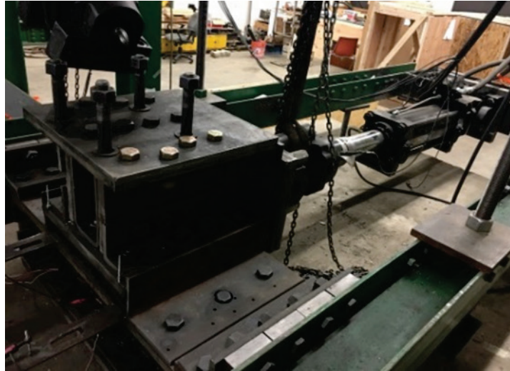
Figure 16. Setup for loosening test.
