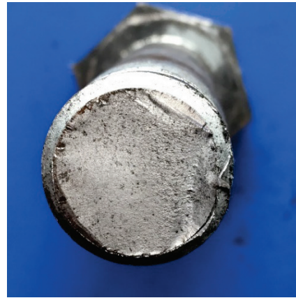
Figure 35. Fractographic profile of specimen #9 (Galvanized 8S_16T N=180070 ).
