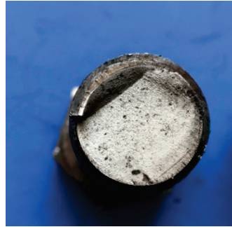
Figure 34. Fractographic profile of specimen #15 (Regular 10S_20T N=228736 ).
