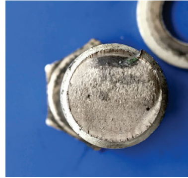
Figure 30. Fractographic profile of specimen #6 (Galvanized 16S_16T N=32,964 ).
