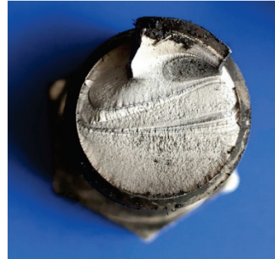
Figure 31. Fractographic profile of specimen #20 (Regular 16S_16T N=53,484 ).
