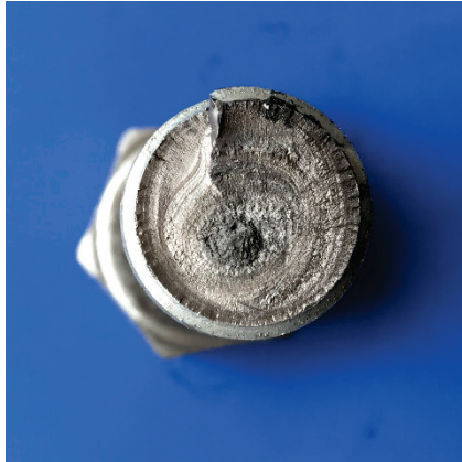
Figure 28. Fractographic profile of specimen #2 (Galvanized 20S_20T N=43,423 ).
