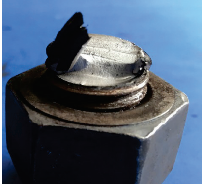
Figure 31. Fractographic profile of specimen #20 (Regular 16S_16T N=53,484 ).
