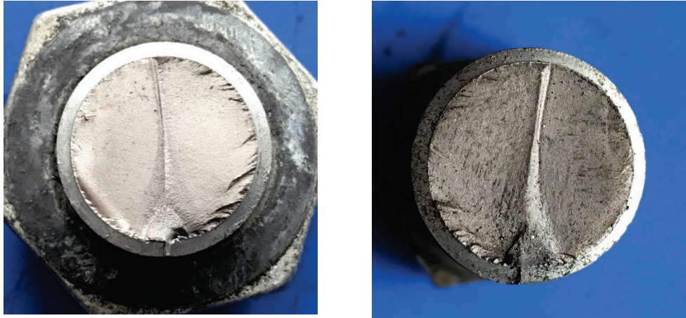
Figure 32. Fractographic profile of specimen #10 (Galvanized 8S_8T N=838,878).
