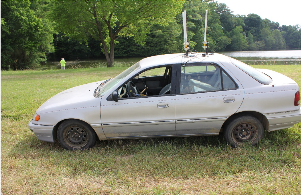
Figure 3. Example of vehicle with remotely piloted vehicle system installed.
