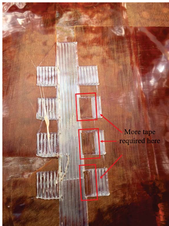
Figure A.1. First layer of raft, areas missing material require more Kapton tape for bed adhesion.
