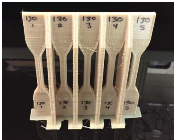
Figure 3.7. ASTM D-638 Type IV tensile specimens printed in the modified TAZ 6.
