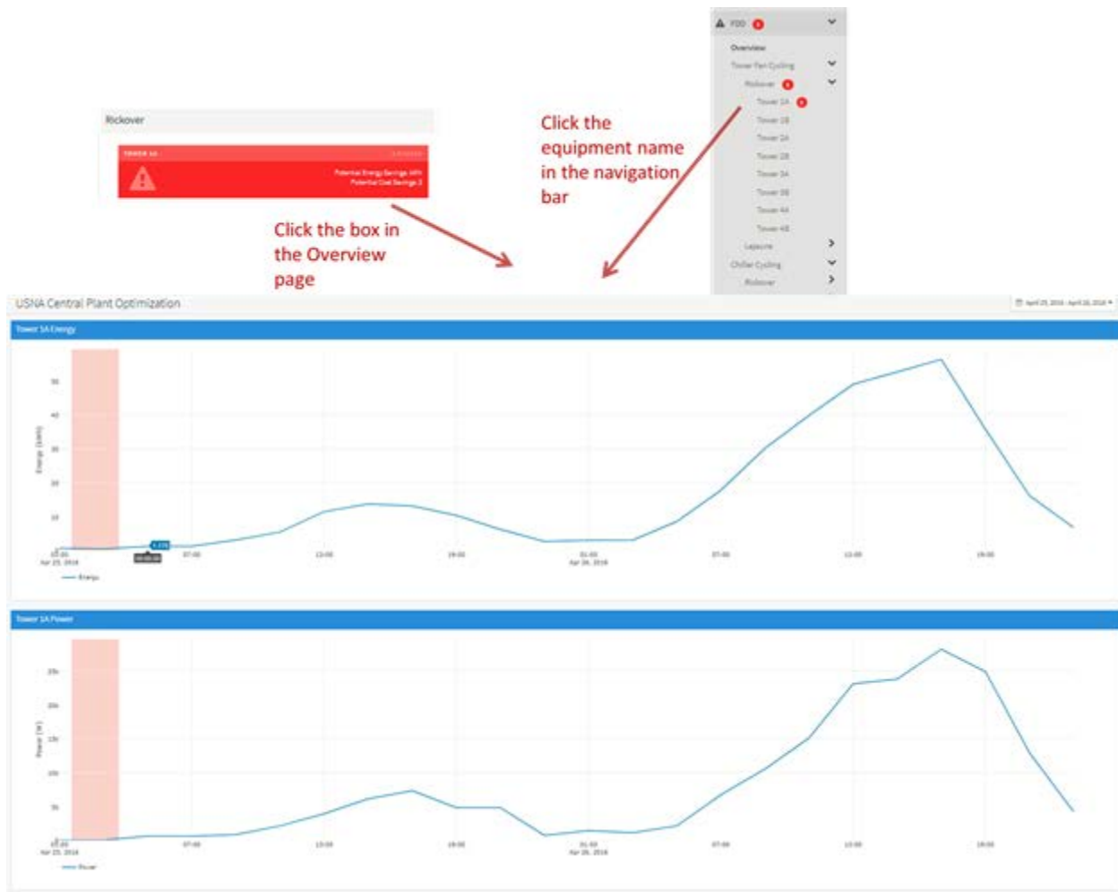
Figure F- 13. The equipment-specific fault drill-down page
