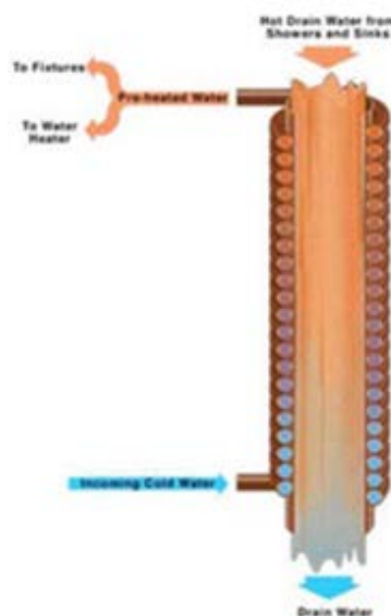
Figure 1. GFX Schematic
