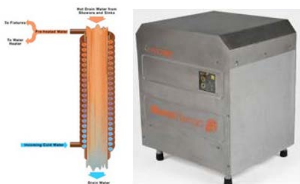
Figure 25. External Waste Water Heat Recovery Methods
