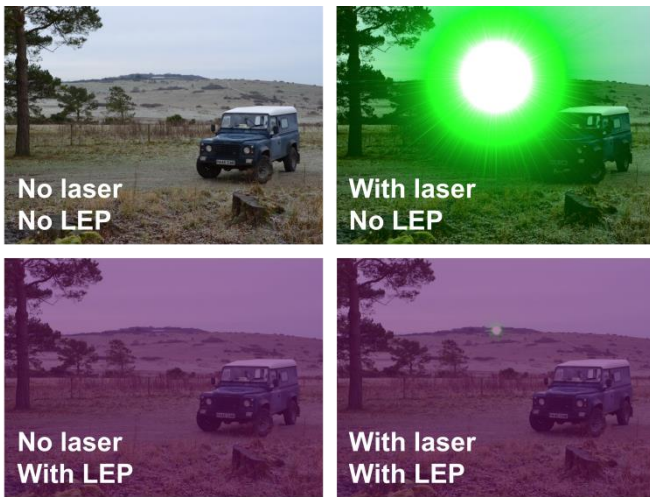
Fig. 5. Simulated representation of the visual impact of wearing LEP, with and without laser exposure. Each image has a scene horizontal field of view of 40°.
