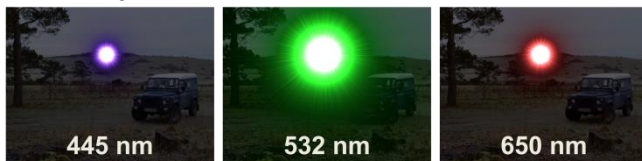
Fig. 4. Simulated images showing human dazzle differences between blue (445 nm), green (532 nm) and red (650 nm) lasers of equal irradiance (50 μW·cm -2 ) at dusk/dawn (10 cd·m -2 ) conditions. Each image has a scene horizontal field of view of 40°.
