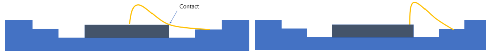
Figure 42. A depiction of a side contact vs. a center one. The side contact is less likely to form a connection with the edge of the chip.
