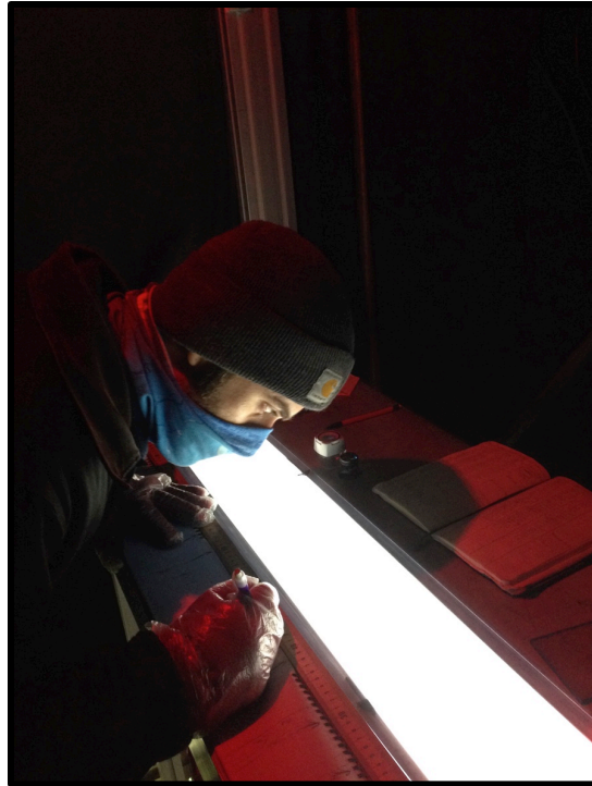
Figure 3. We observed the physical properties of the illuminated cores within the dark booth as shown and recorded their respective depth offsets in paper log books.
