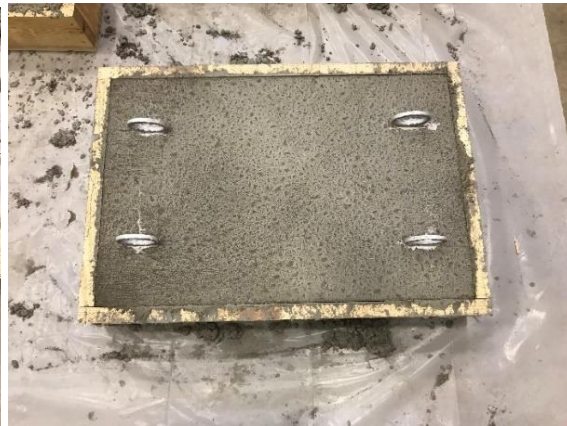
Figure 15. Finished Slab Specimen
