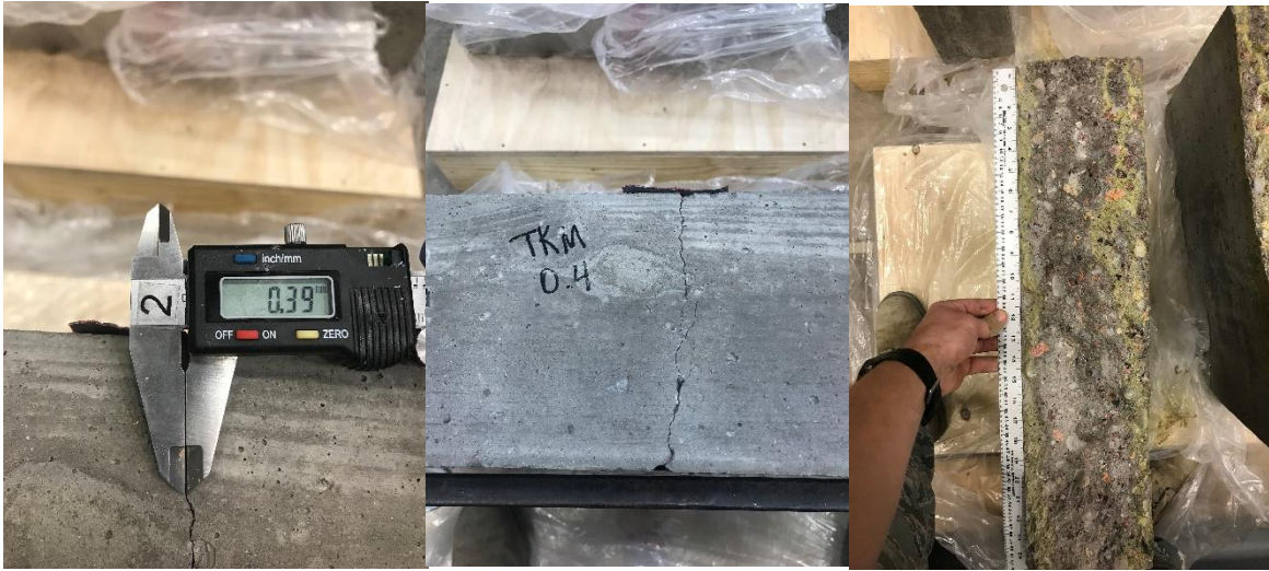
Figure 33. TK-2415 Slab Specimen at 0.4 mm
