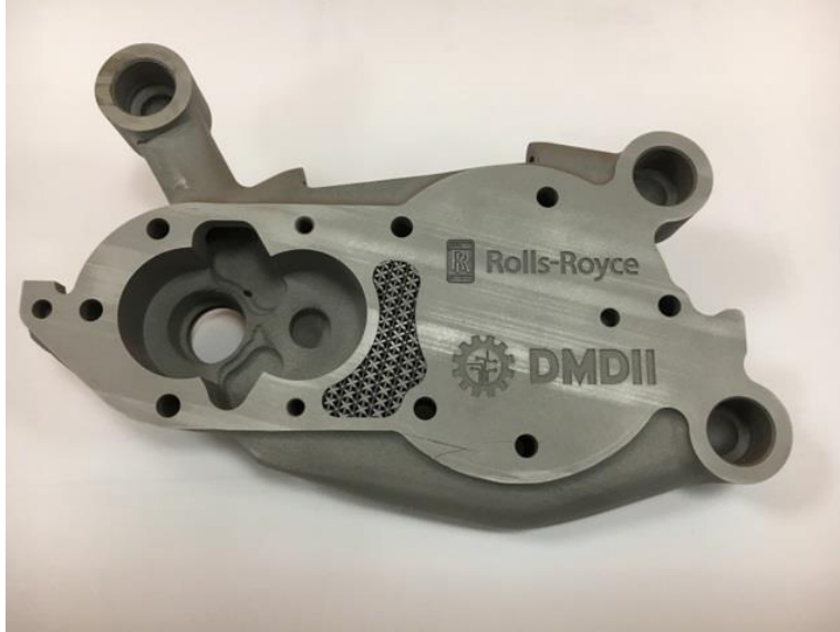
Figure 17: Additive Manufacturing of Pump Body Housing
