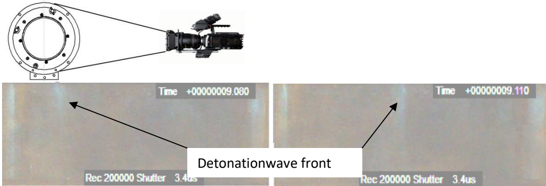
Fig.11. Screenshots from high speed record of the shock-wave motion. The camera was positioned relative to the combustion chamber.
