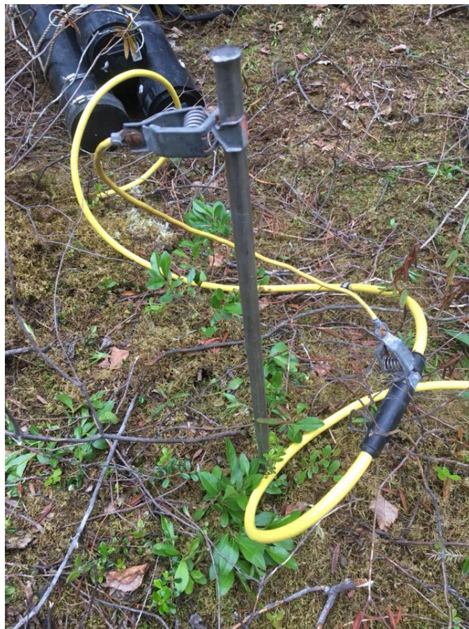
Figure 3.7: Standard ERT Probe Configuration
