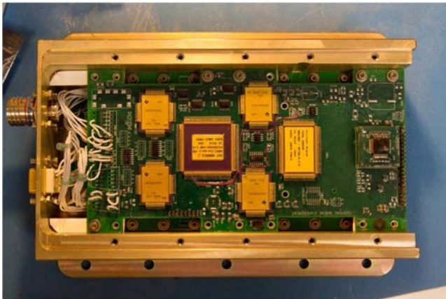
Fig. 2. RHEME instrument with lid removed
