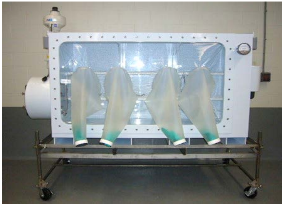
Figure 3. Close-up View of Semi-Rigid Germ-Free (GF) Isolator
