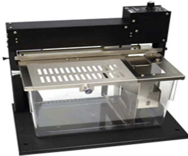
Figure 13. Sleep Fragmentation Chamber from Lafayette Instruments (Lafayette, Indiana)
