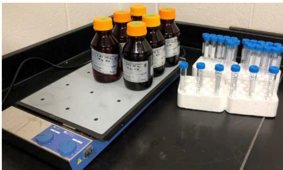
Figure 12. Solutions containing 5 ppm BB and MB dye solution being stirred prior to adding carbon for the experiments.
