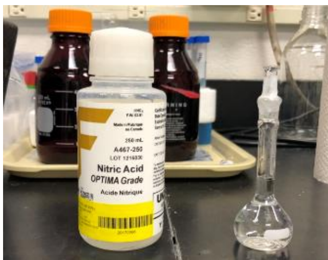
Figure 5. The Optima Grade Nitric Acid being mixed to create the electrolyte solution used in the electrochemical modification of the carbon materials.
