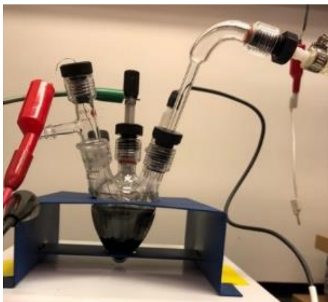
Figure 7. The electrochemical cell used in the modification of virgin GAC and CNF.
