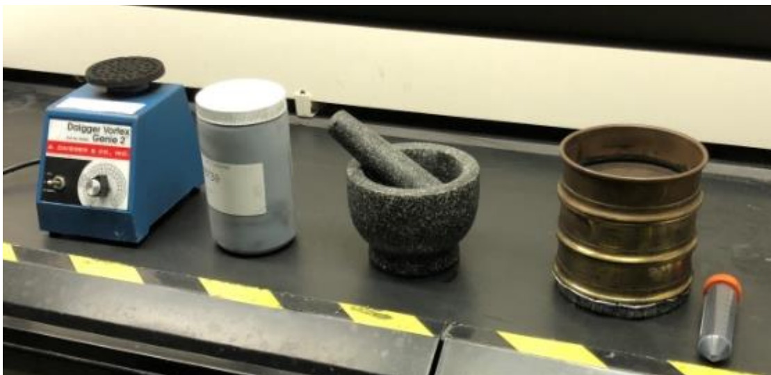
Figure 6. The tools (mortar, pestle, sieves, and shaker) used to crush and sieve.
