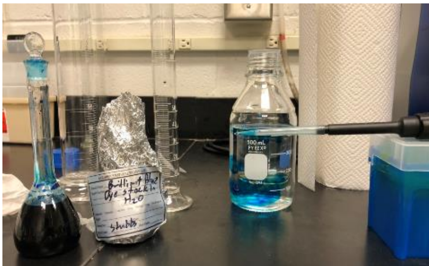
Figure 1. The Brilliant Blue dye (BB) dye shown mixed during pilot study to determine the amount of GAC to be used in future experiments.
