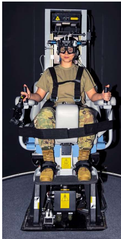
Figure 2. RC with VOG goggles and restraints.
