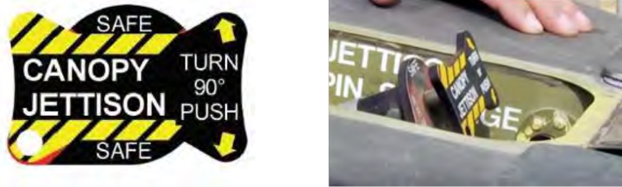
Figure 185. Exterior side canopy jettison handle on AH-64D.
