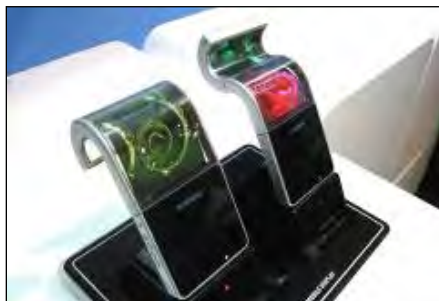
Figure 76. Flexible display capability of AMOLED technology (Source: Samsung).
