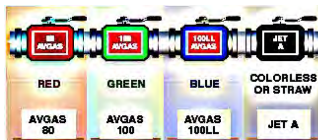
Figure 191. Color code for aviation fuel.
