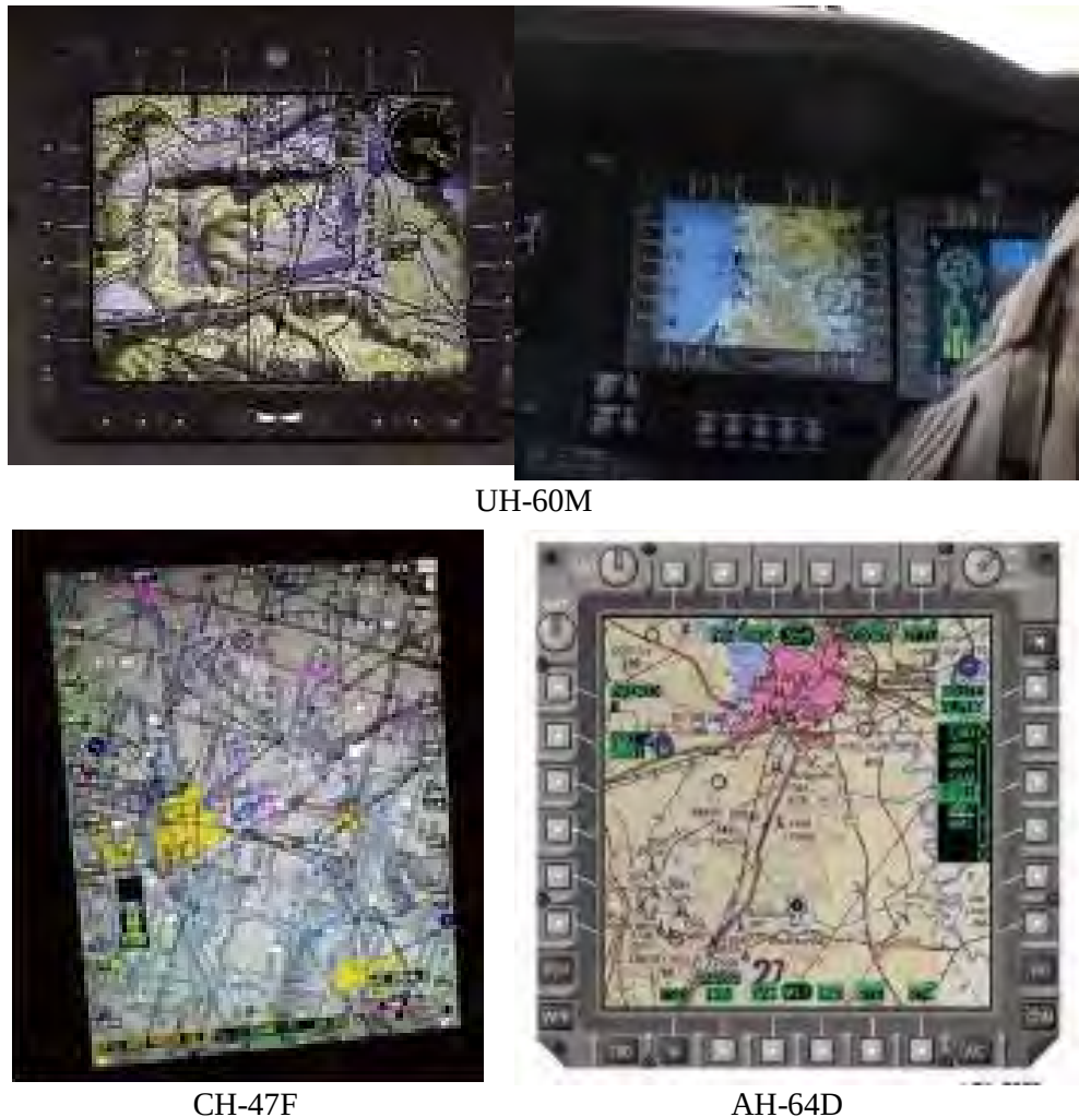
Figure 118. UH-60M (top), CH-47F (bottom, left), and AH-64D (bottom, right) digital moving map displays.
