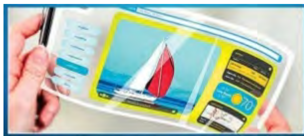
Flexible and transparent OLED display
