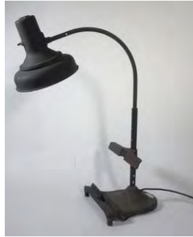
Figure 161. The MacBeth easel lamp used for many PIP color vision tests.
