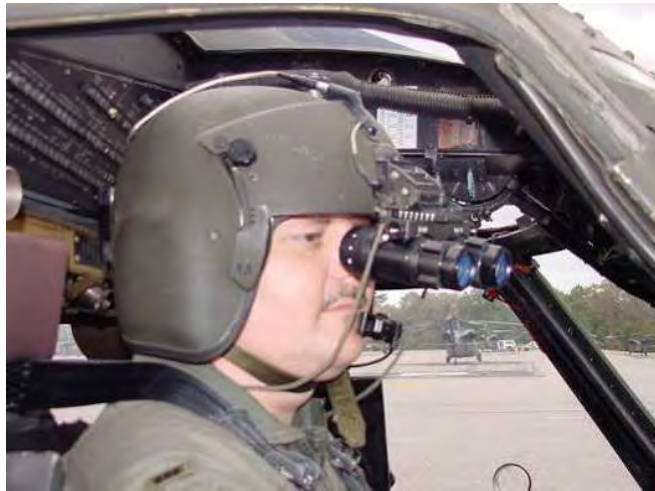
Figure 170. The AN/AVS-6 Aviator’s Night Vision Imaging System (ANVIS).
