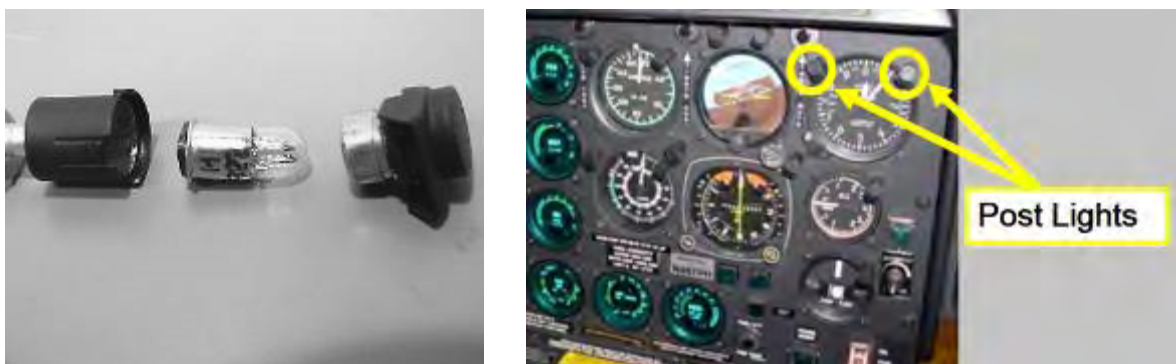
Figure 13. Post light showing an incandescent bulb mounted in a cylinder. 68
