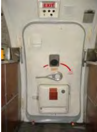
Figure 99. Examples of emergency exit locking mechanism marking and emergency exit locator sign in passenger aircraft.
