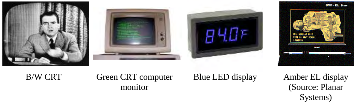
Figure 71. Examples of monochrome (single color) displays.
