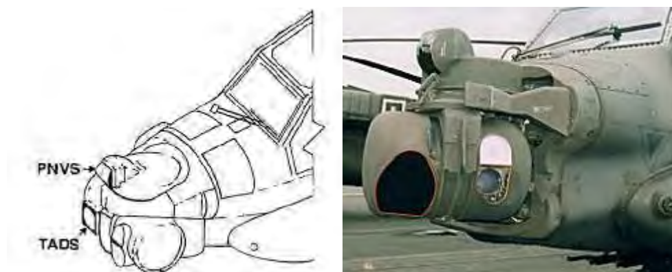
Figure 164. The nose-mounted PNVS and TADS FLIR sensors on the AH-64 Apache helicopter.
