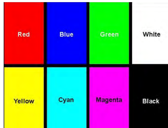
Figure 112. Recommended colors for avionics displays (Cardosi & Hannon, 1999).
