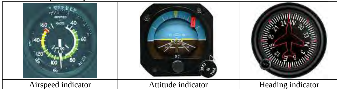
Figure 110. Examples of color in fixed cockpit instruments.
