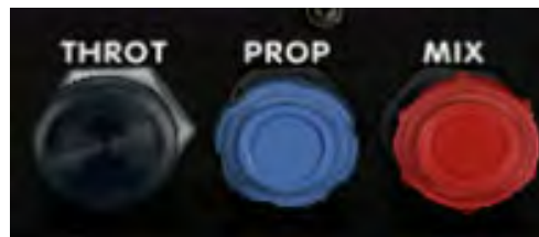
Figure 101. Color coding of engine controls in piston engine aircraft.
