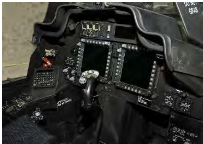
Pilot rear seat: full instrument panel
