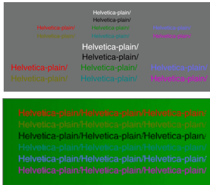
Figure 107. Examples of illegibility where a large hue difference exists, but luminance contrast is small (NASA Ames Research Center, 2000b).
