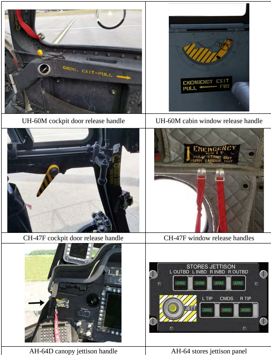
Figure 100. Emergency exit release handles: UH-60M cockpit door (top, left) and cabin window (top, right); CH-47F cockpit door (middle, left) and window ramp (middle, right); and AH-64D canopy jettison (bottom, left) and stores jettison (bottom, right).
