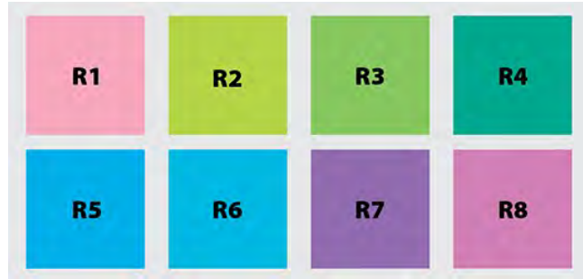
Figure 48. Test colors used in calculating CRI.
