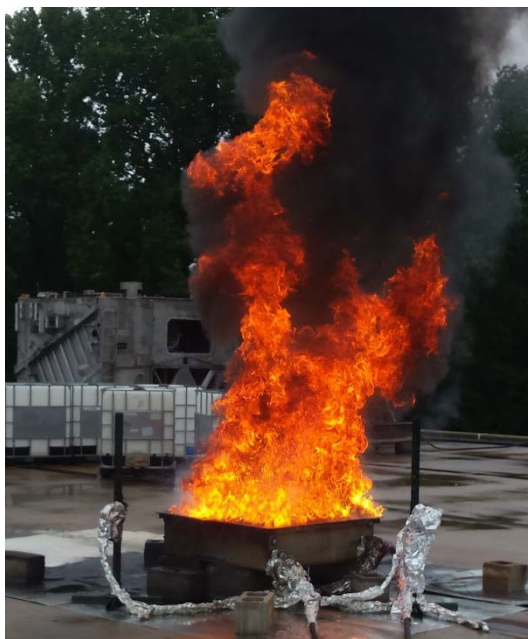
Fig. 14-Typical ISB pan fire of Santa Ynez crude oil. There was steam around the edges of the pan as the flames heated the water through the oil.
