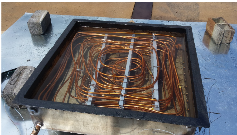
Fig. 3-1 m 2 -square burn pan with heat exchanger coils and thermocouples installed.
