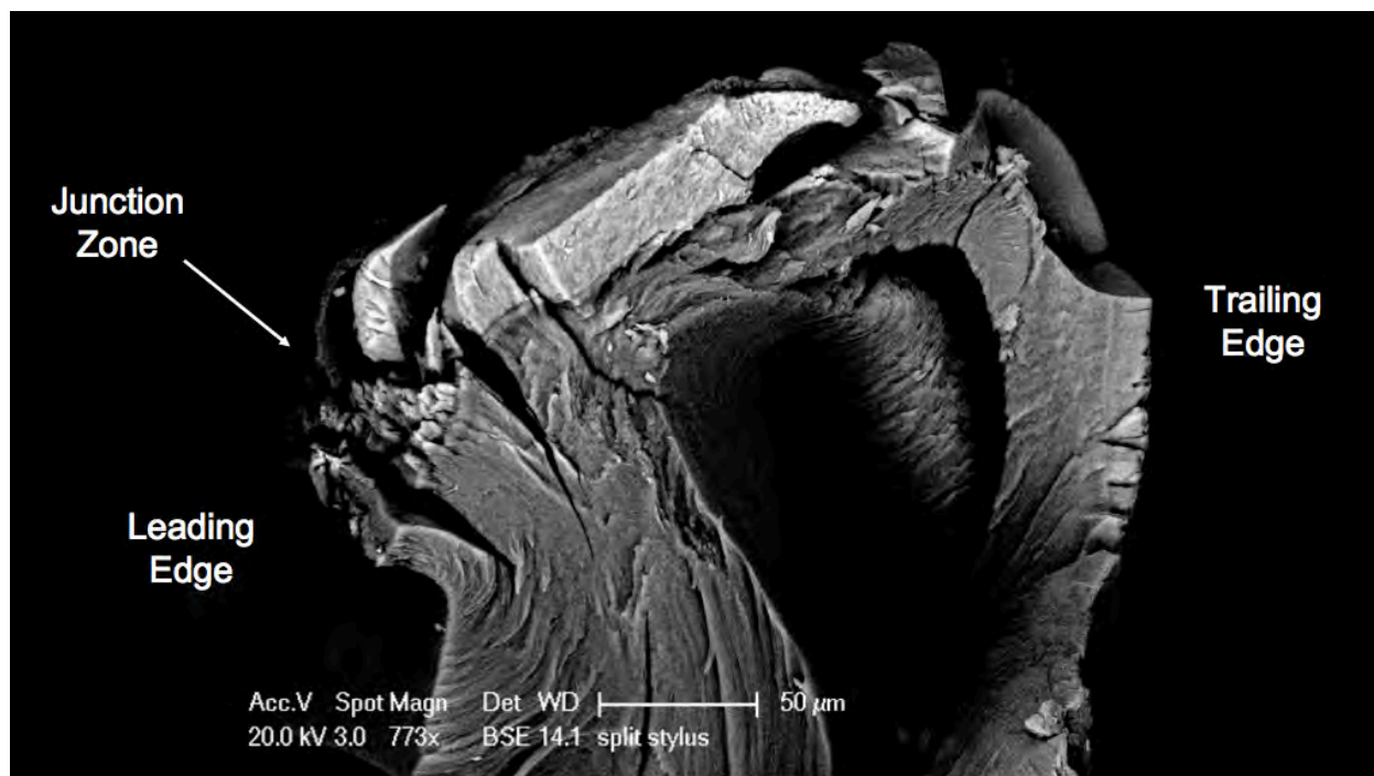
Figure 32. Back-scattered scanning electron micrograph of fractured stylus highlighting mineral interface.
