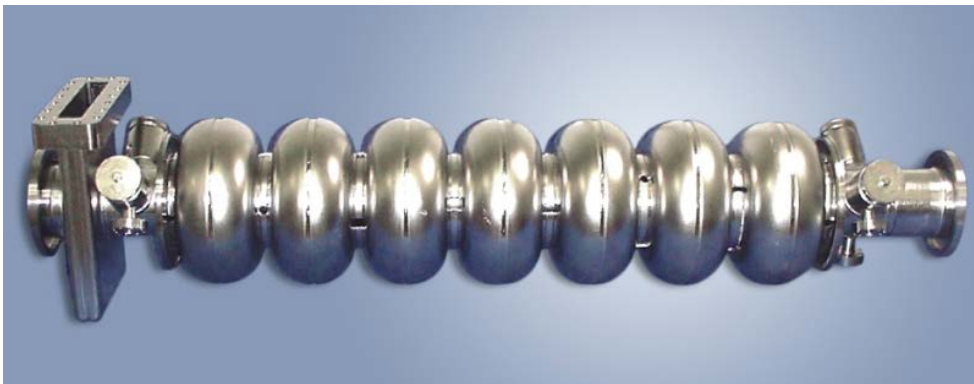
Figure 2. A niobium accelerator cavity. The function of the accelerator cavity is to increase electrons' energy from low (~5 MeV) to high (~100 MeV) through the alternating electric fields. From [4].
