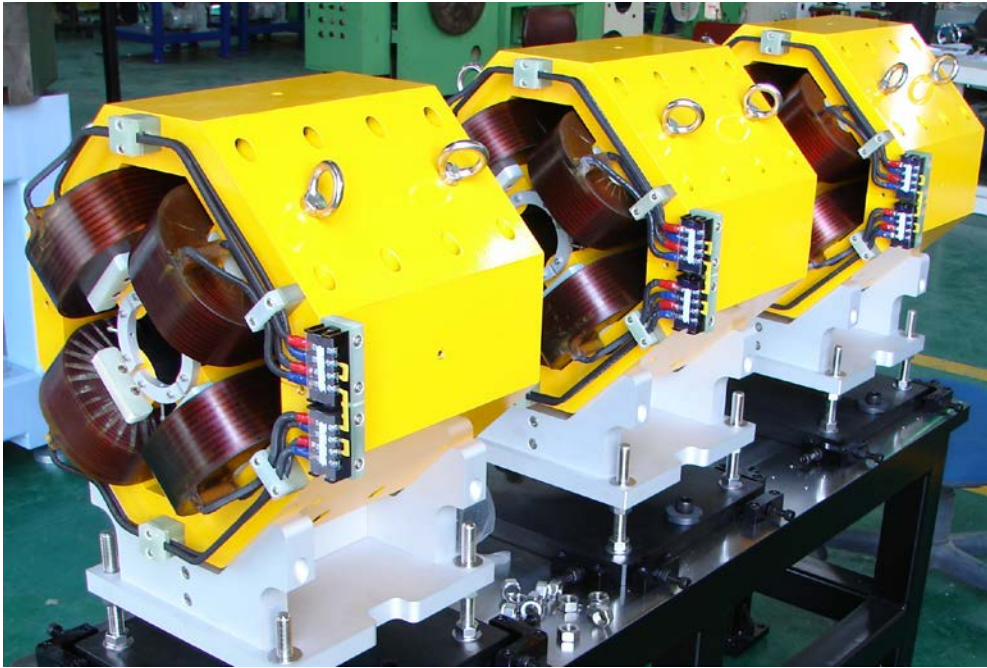
Figure 8. A quadrupole triplet. Focusing characteristic makes quadrupole magnet a significant component in an FEL beamline. The four brown coils mounted on yellow shell create quadrupole magnetic field to focus electrons. A long FEL beamline consists of many sets of quadrupole doublet or triplet of quadrupole for the sake of maintaining transporting electron within the beam pipe. From [7].
