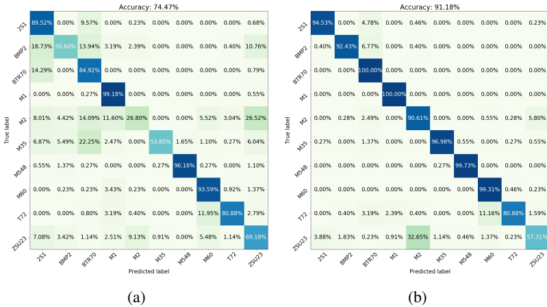
Figure 1.10: Confusion matrices corresponding to S^{12345}M^1S^{2345} (a) and M^{12345}M^{123}S^{45} (b). The weighted accuracy for the withheld T72 and ZSU23 classes in (a) is 73.4%, and the weighted accuracy in for the same two classes in (b) is 65.9%.
