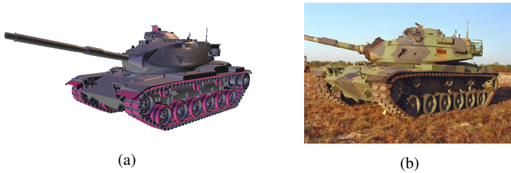
Figure 1.2: An AFacet CAD model of a M60 tank (a) that has gone through the iterative validation process described here. The image in (b) is one of the collected images with which the CAD model was compared. Note the correct position of large elements, such as the turret, and small elements, such as various hatches.
