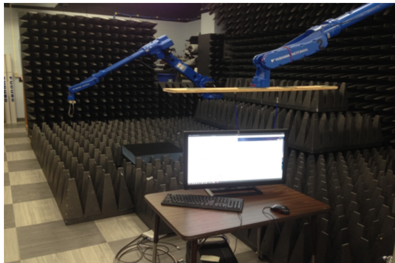
Figure 4.6: Test Configuration 1 Semi-Anechoic Chamber in the Mumma Lab
