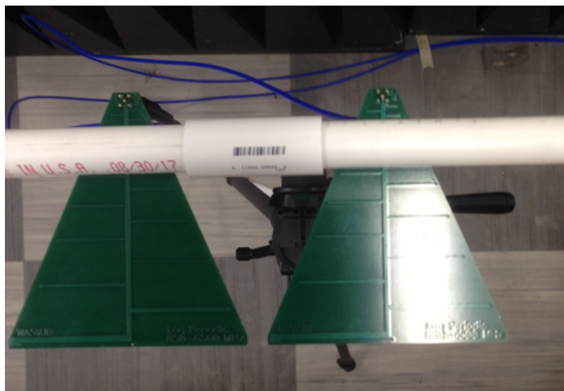
Figure 4.2: Original Mount for Two Antennas with 15 cm Spacing
