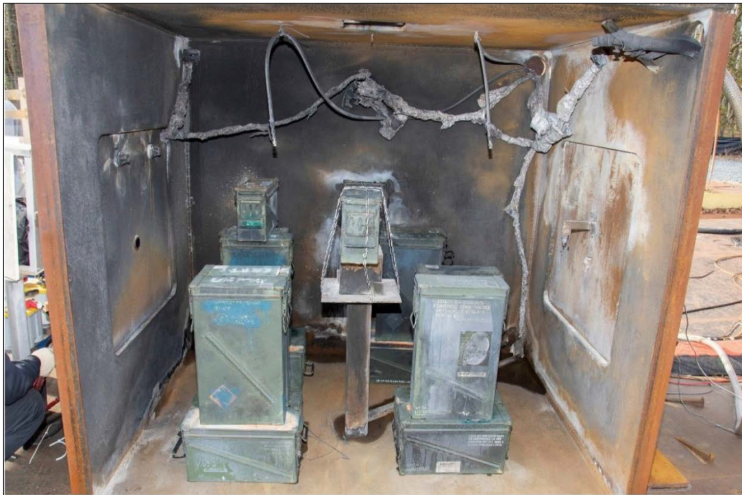
Figure 2.8-2. Test chamber (172 ft 3 ) with clutter (simulated with ammo cans) and side panel removed.
