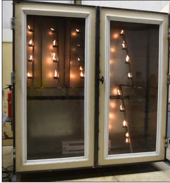
Figure 2.5-3. ATC hidden fire test chamber.
