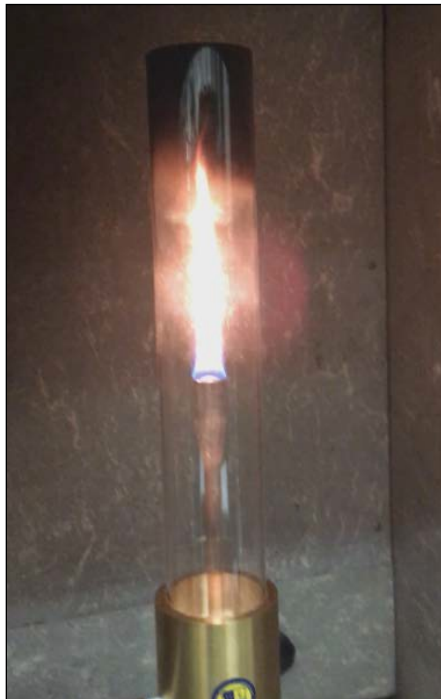
Figure 2.4-4. Sub-scale (5/8) experimental setup to quantify agent extinction concentrations.
