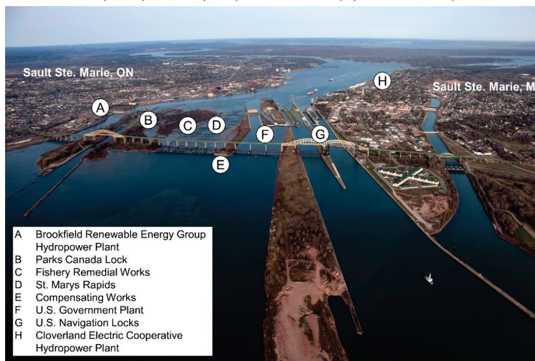
Figure 2. Hydropower and other control structures on the St. Marys River connecting Lake Superior (bottom of photo) and Lake Huron (top, in the distance).
