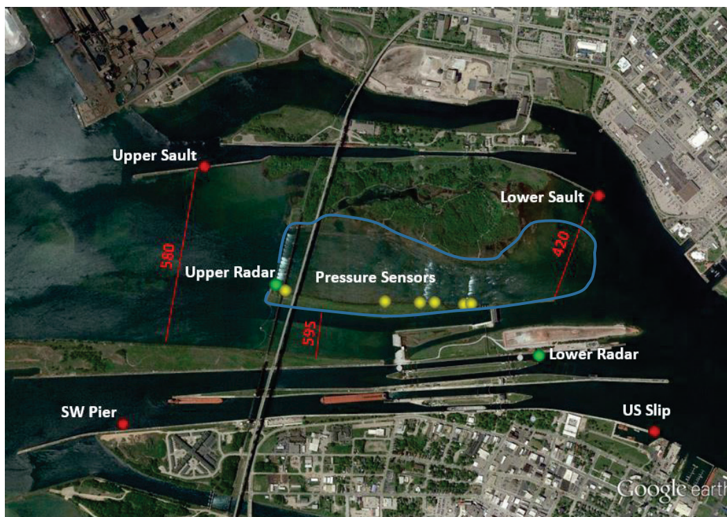
Figure 5. St. Marys rapids (outlined in blue) with pressure sensor locations (yellow dots, sensor 1 is most upstream), radar gauge locations (green dots), NOAA or CHS gauging locations (red dots) and discharge measurement locations (red lines).
