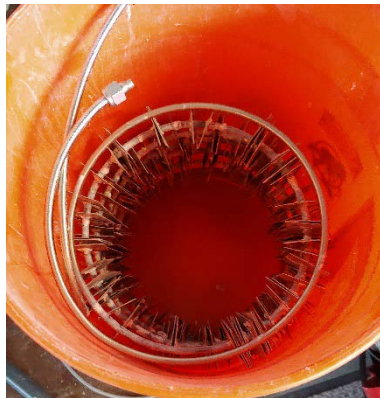
Figure 5. Ice-Water Heat Exchanger
