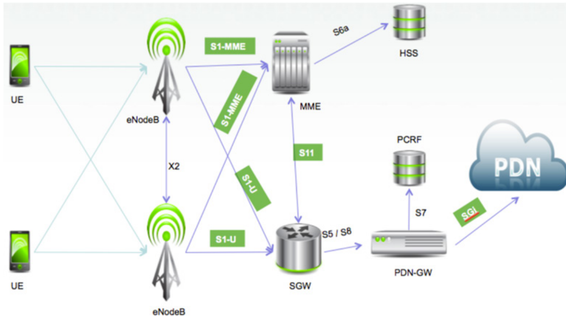
Figure 41. Diagram of 4G Network. Source: InteliSecure (2019).
