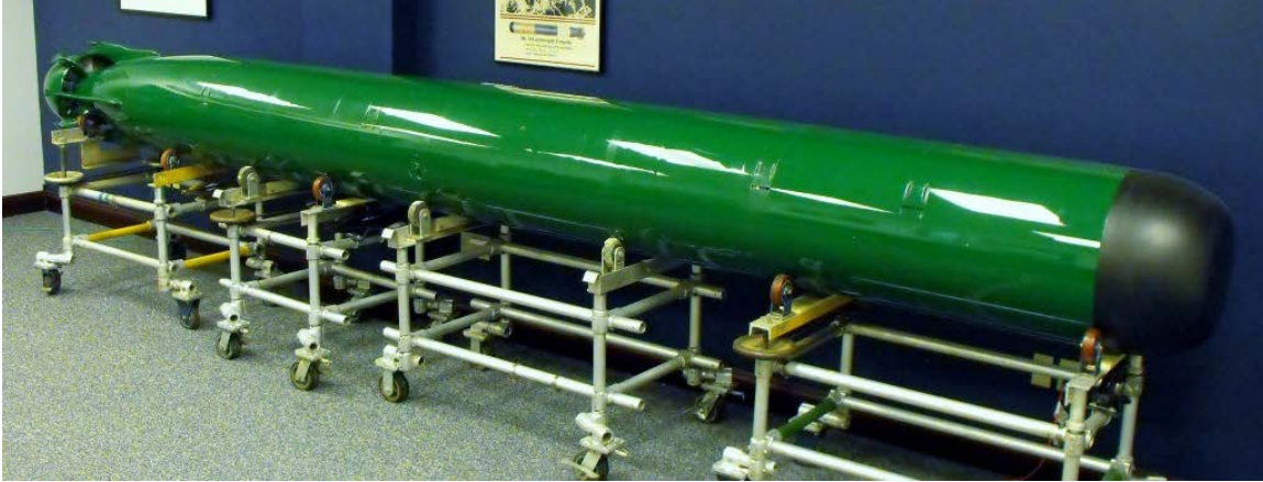
Figure 18. MK 48 Heavyweight Torpedo on Maintenance Carts. Source: Ordnance Technology Services (n.d.).
