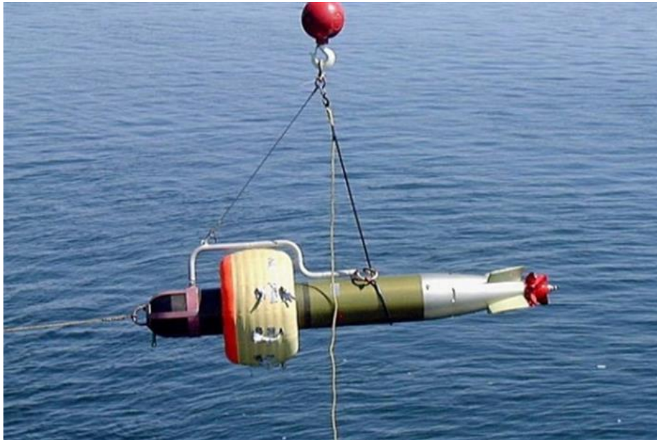
Figure 17. Recovery of MK54 Lightweight Torpedo Using an Over-the-Side Crane. Source: C4 Defence (2018).
