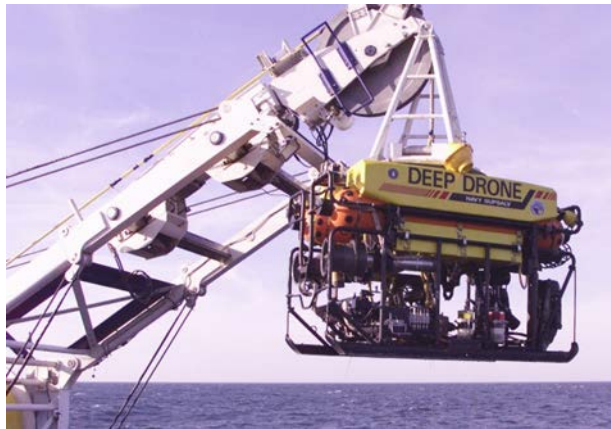
Figure 19. Launching of Remotely Operated Vehicle from Unknown Vessel. Source: NAVSEA (n.d.).
