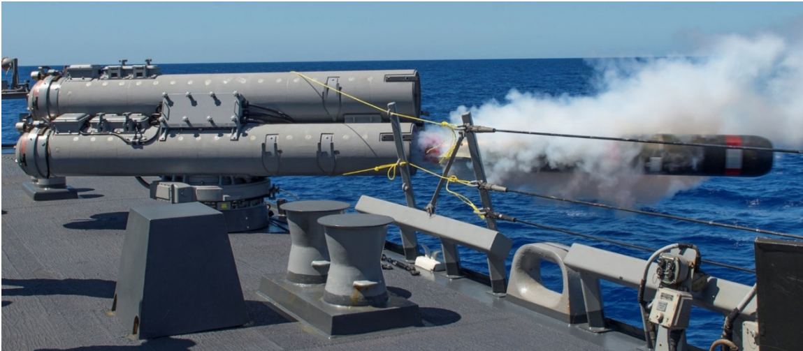
Figure 16. MK32 Surface Vessel Torpedo Tube Launching an MK46 Lightweight Torpedo. Source: Seaforces-Online (n.d.).
