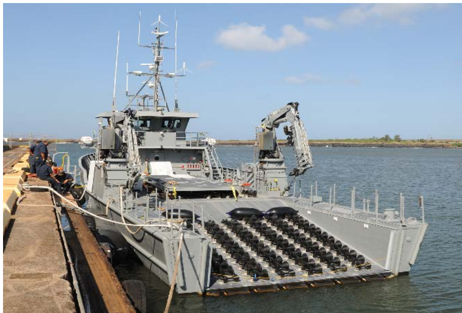
Figure 24. MPC-2 Docked at PMRF Showing Stern Ramp and Cranes. Source: Within Range (2014).
