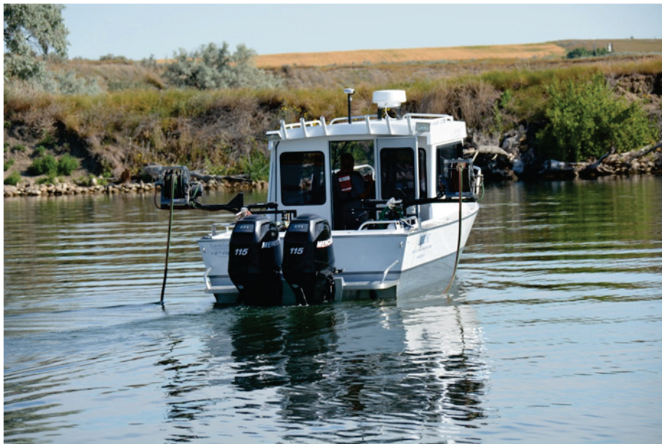
Figure 6. Variable depth LittLine® application of herbicide and rhodamine WT dye on 23 September 2014.
