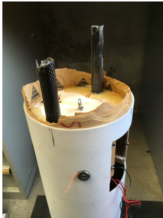
Figure 34. Broken Booster-Sustainer Coupler
