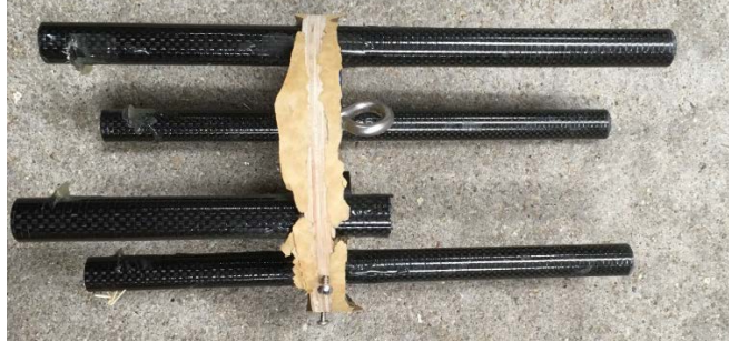
Figure 37. Broken Booster-Sustainer Coupler
