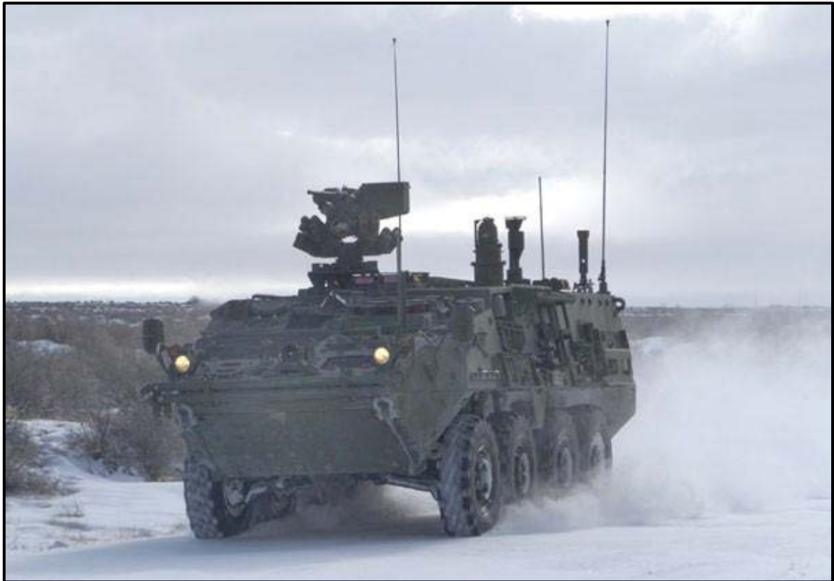
Figure 3. Stryker Nuclear, Biological, and Chemical Reconnaissance Vehicle configuration (a vehicle with ColPro capability).
