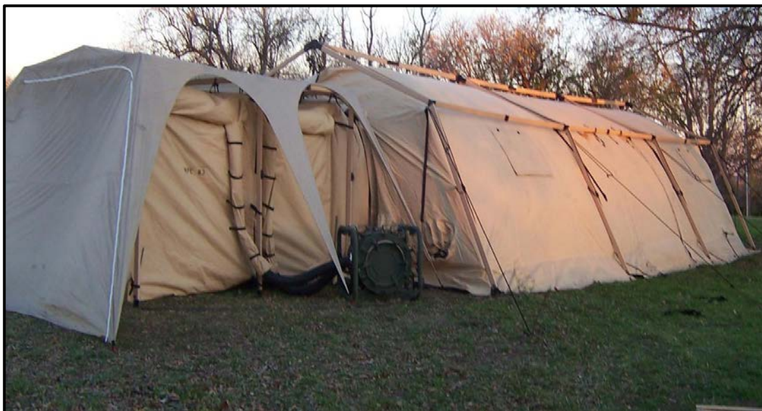
Figure 1. An active ColPro shelter with airlock and GPFU.
