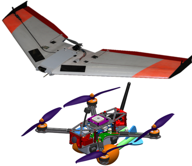
Figure 4.1. The two UAV airframes that we used in our implementation: the Zephyr II fixed-wing is depicted in the top image and the Mosquito Hawk quadrotor is depicted in the bottom image.
