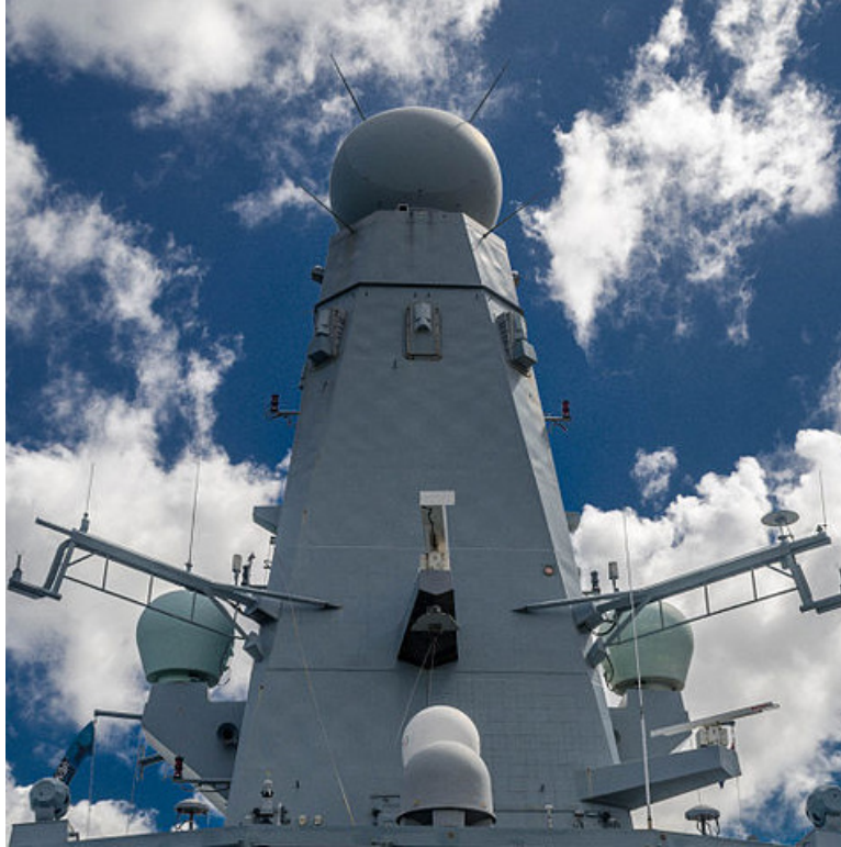
Figure 9. SAMPSON Radar (Radome Atop Mast). Source: Hpeterswald (2013).
