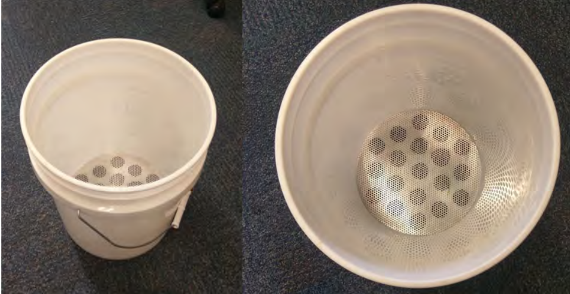
Figure 12. Ice Bucket Showing Perforated False-Bottom
