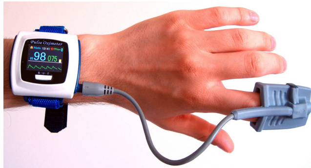
Fig. 1 Finger cuff pulse oximeter. Wrist monitor shows blood oxygenation, pulse rate, and PPG signal. (Wikimedia Commons contributors. File:Wrist-oximeter.jpg. Wikimedia Commons, the free media repository; 2018 Nov 27, 15:59 UTC [accessed 2019 July 29]. https://commons.wikimedia.org/w/index.php?title=File:Wrist-oximeter.jpg&oldid=329545296. )
