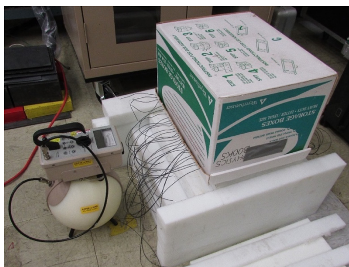
Figure 52. Shielded Sensors Exposed to PuBe Source
