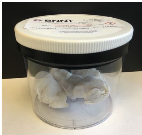
Figure 31. BNNTs as Received from BNNT, LLC
