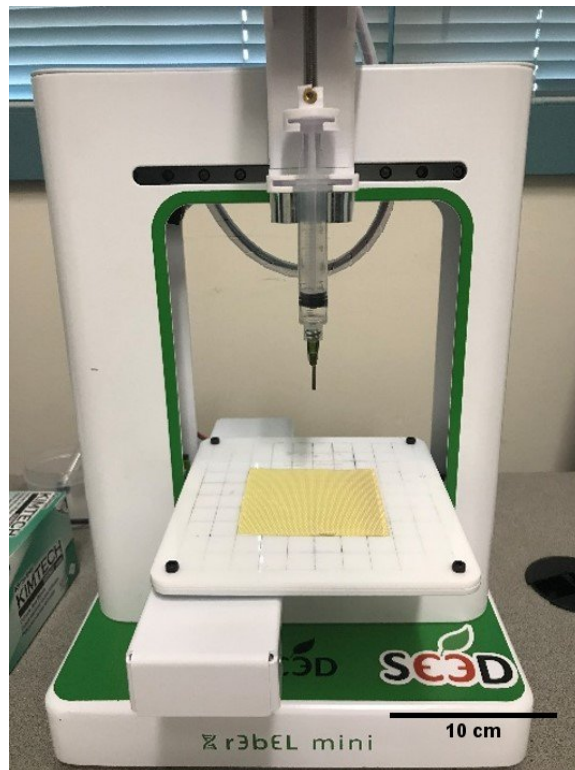
Figure 9. SE3D Rebel mini gel 3D printer setup.
