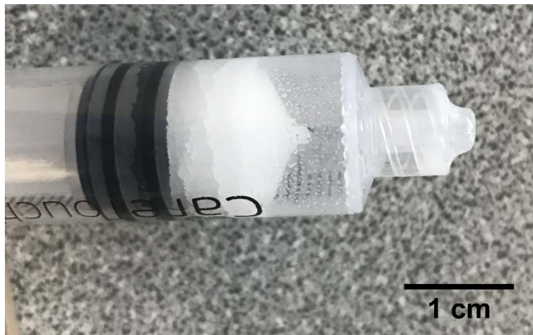
Figure 25. Segregated carbopol and PCM after printing attempt.
