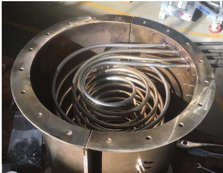
Figure 3. Modified Heat Exchanger
