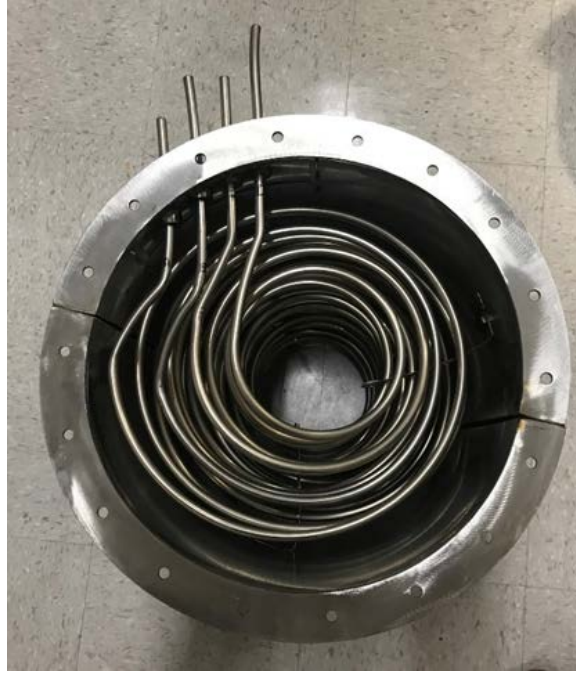
Figure 2. Previous Heat Exchanger Design
