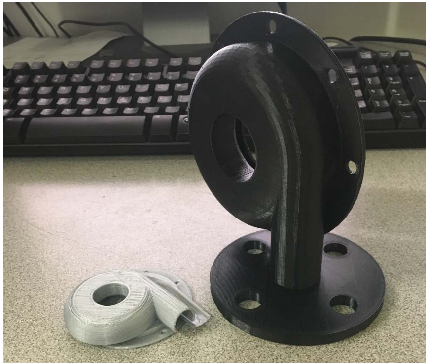
Figure 14. Final 3D Printed Volutes (Right) and Half-Scale Volute (Left)
