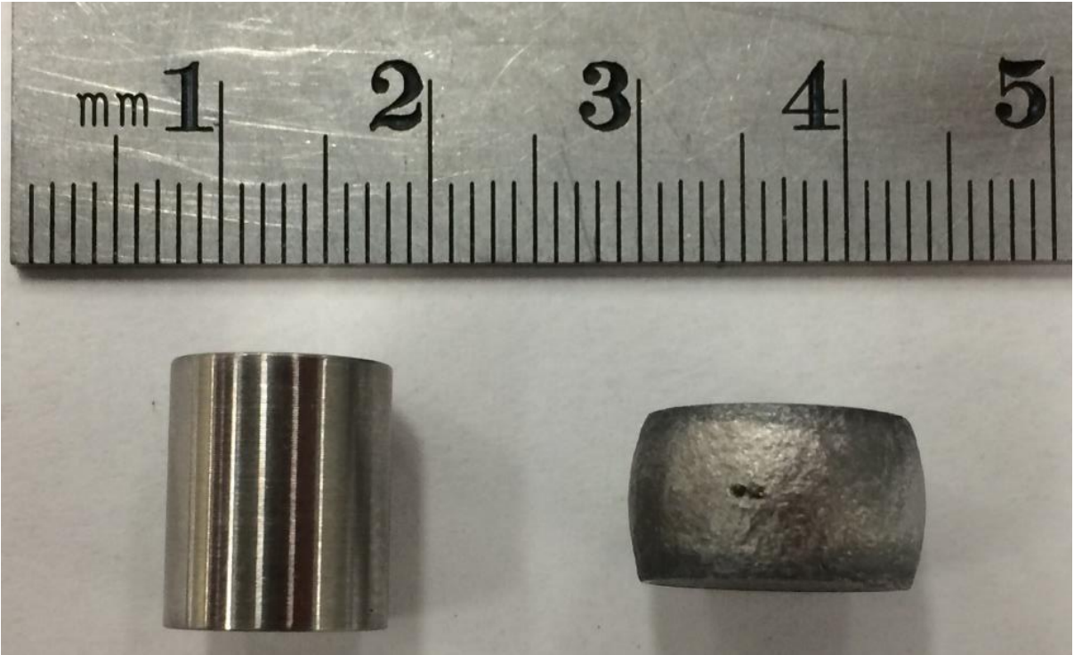
Figure 1. Examples of the specimen before and after compression testing.
